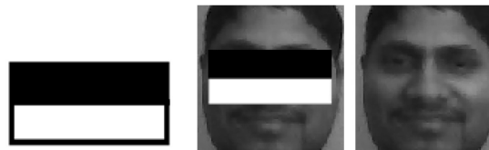
Haar Feature that looks similar to the eye region which is darker than the upper cheeks is applied onto a face
