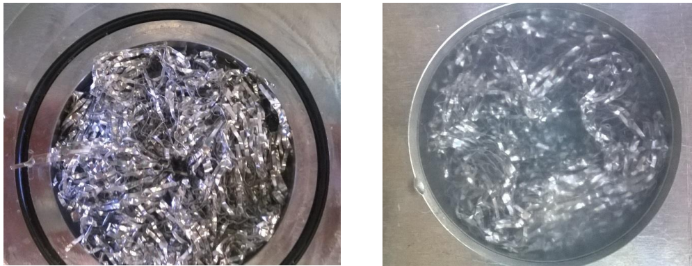
Figure 32 – Explosafe frontal view inside the tank (without and with ionomer panel respectively)
