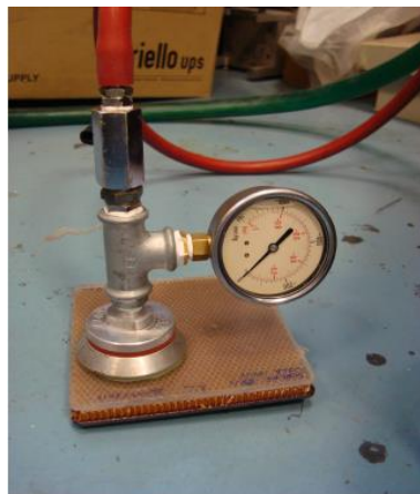
Figure 37 – Leakage test instrument.
