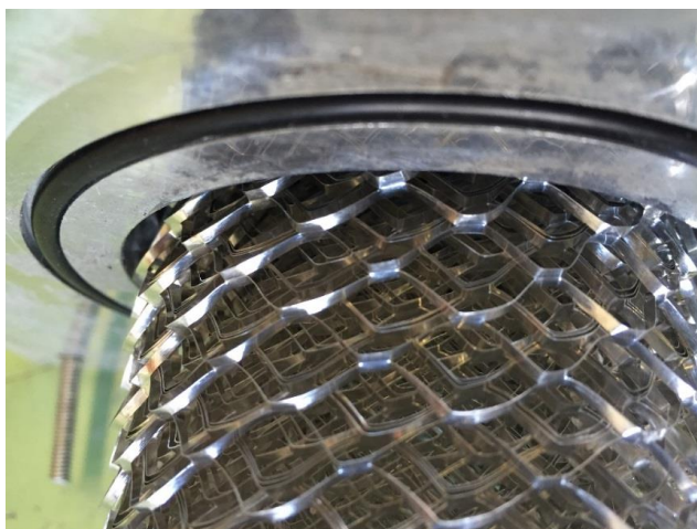
Figure 33 – Explosafe insertion phase inside the experimental tank.
