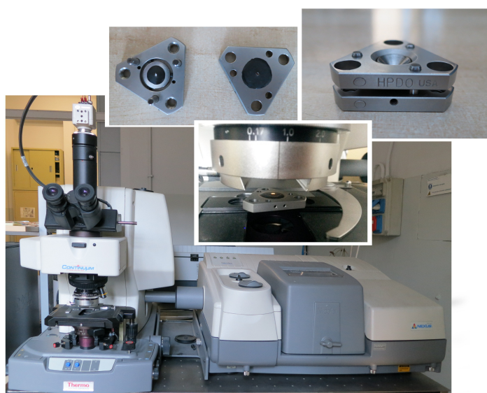
Figure 3.8. FT-IR instrumentation with the Diamond Anvil Cell used for the analyses.
