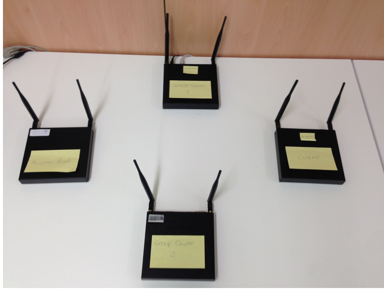
Figure 5.8: Four alix connected through three different P2P groups.
