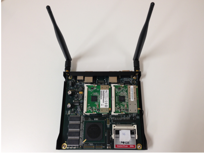
Figure 5.3: Alix Board composed by two wireless interfaces.
