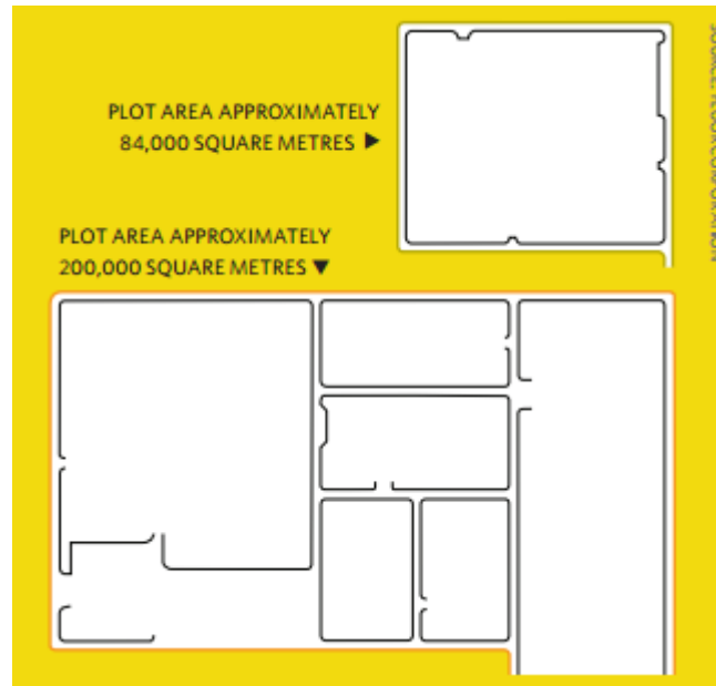
Figure 7 – In situ facility plot size reduction (Fluor Corporation)
