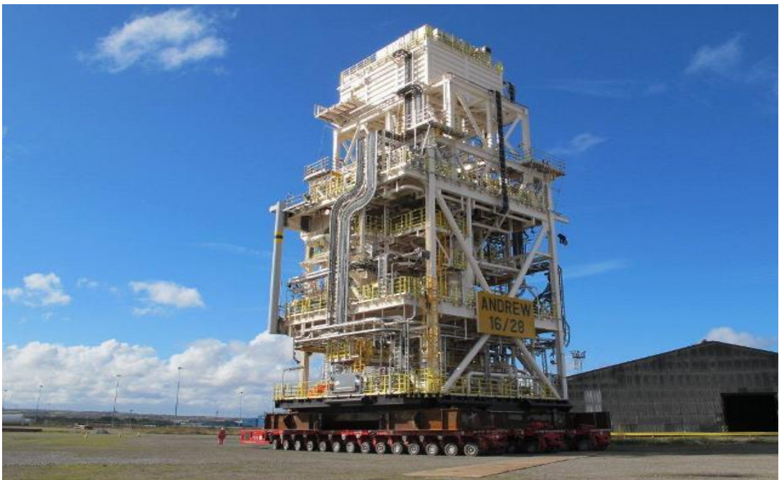
Figure 5 - Equipment or process module
