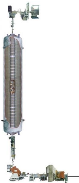
Figure 6.1: the 14UD pelletron accelerator at the Heavy Ion facility at the Australian National University (ANU).
