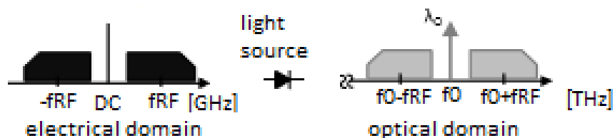
Figure 3.11: IMDD signal E/O spectrum in the electrical and optical domains
