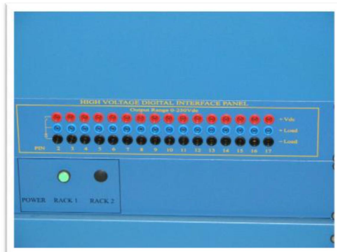
Figura 3.6 Pannello “High Voltage Interface Panel”.
