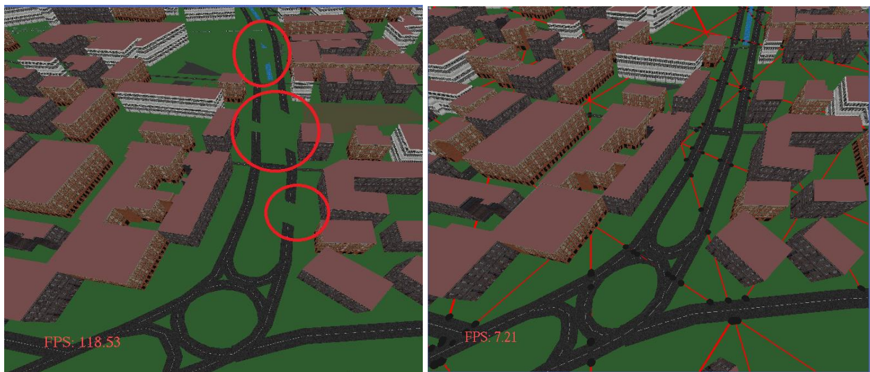
Figure 3.38 – (a) Road with Height Map visibility Problem (b) Draped Highway with pin Points
