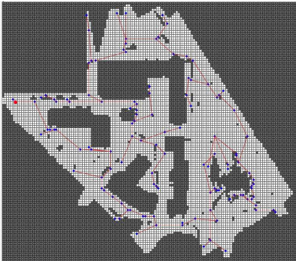
Figure 5.1: Sensing positions identified during the exploration of the Freiburg University's map using Configuration K, 15 meters for the gas sensor range and 180 degrees for the scan angle \phi .
