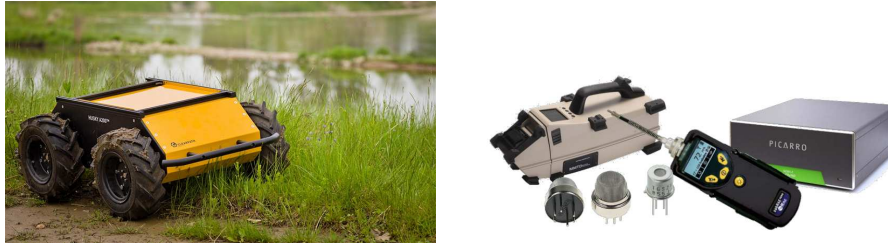
Figure 2.1: Because the flexibility they can offer, mobile robots (left) represent an important innovation in a dangerous task like the gas detection one. In the first years they were combined with in-situ gas sensors (right), whose limitation is the fact they have to be in direct contact with the gas to perceive it.
