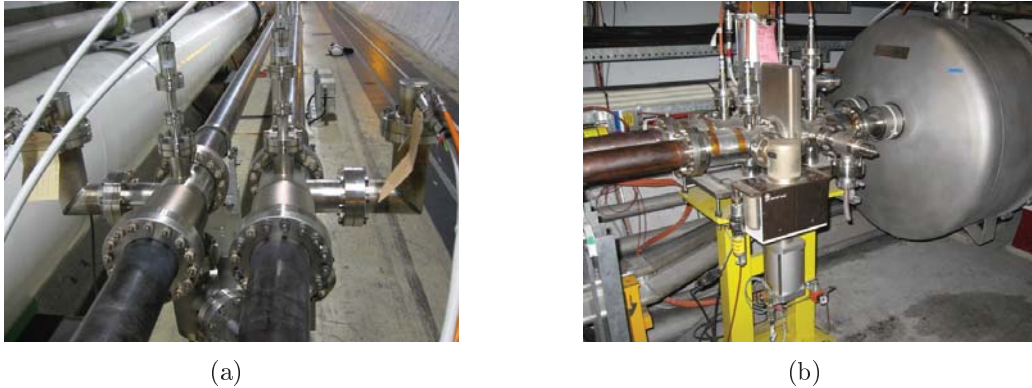
Figure 1.3: A room temperature sector (a) and a warm-cold transition (b). In figure (b) is possible to see the end of the room temperature chamber and the beginning of the cryostat.
