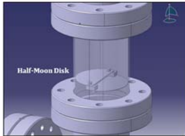
Figure 5.13: Half-moon baffles installed at the gauge port.
