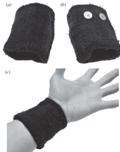
Figure 1. Wearable EDA sensor. (a) Sensor is inside stretchy breathable wristband. (b) Disposable Ag/AgCl electrodes attached to the underside of the wristband. (c) The EDA sensor can be worn comfortably for long periods of time.
