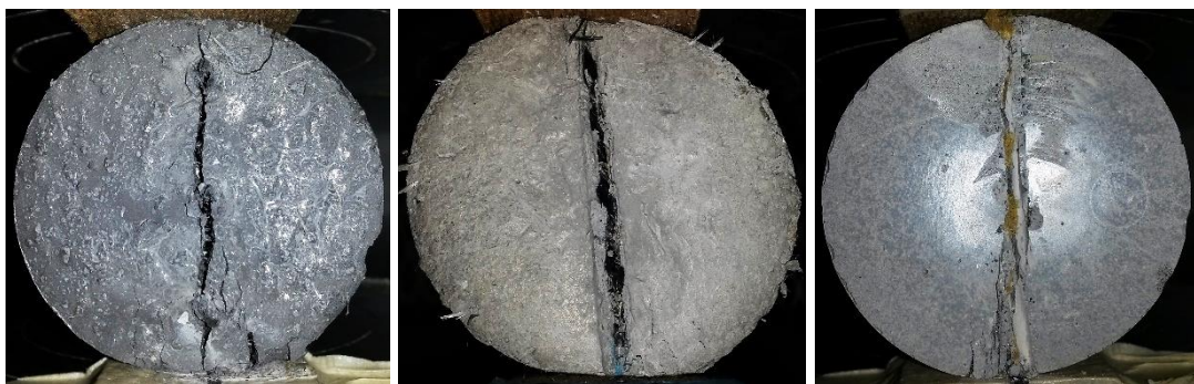
Figure 4.43 – Typical failure modes of cylindrical FRCM specimens
