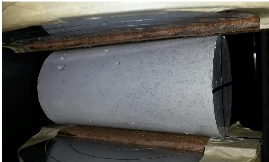
Figure 4.39 – Arrangement of particle wood bearing strips in the machine fixture
