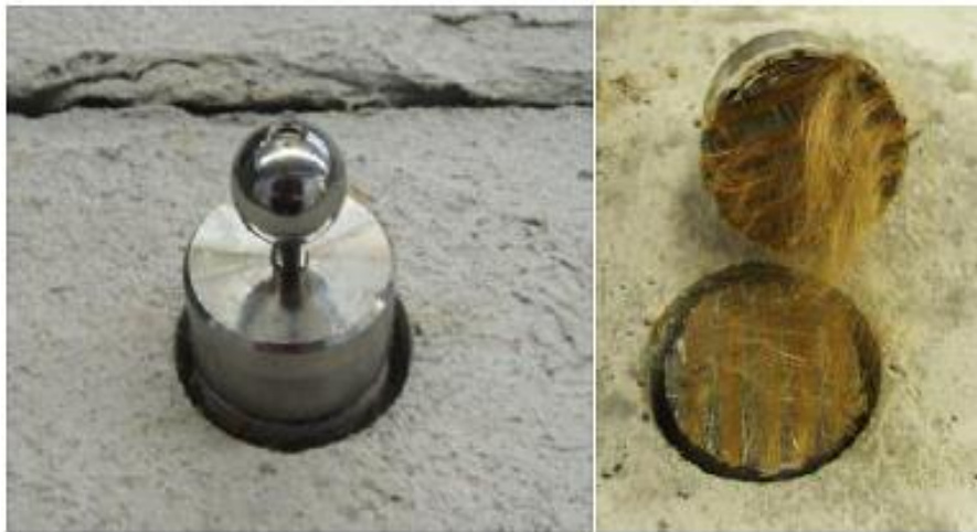
Figure 2.18 – Failure on the interface between the first and the second layer of mortar
