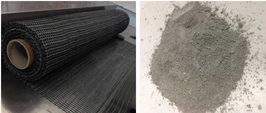
Figure 2.1 – Carbon 1 fabric roll and inorganic cementitious material
