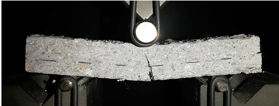
Figure 4.9 - Typical failure mode for one-ply Carbon 2-FRCM
