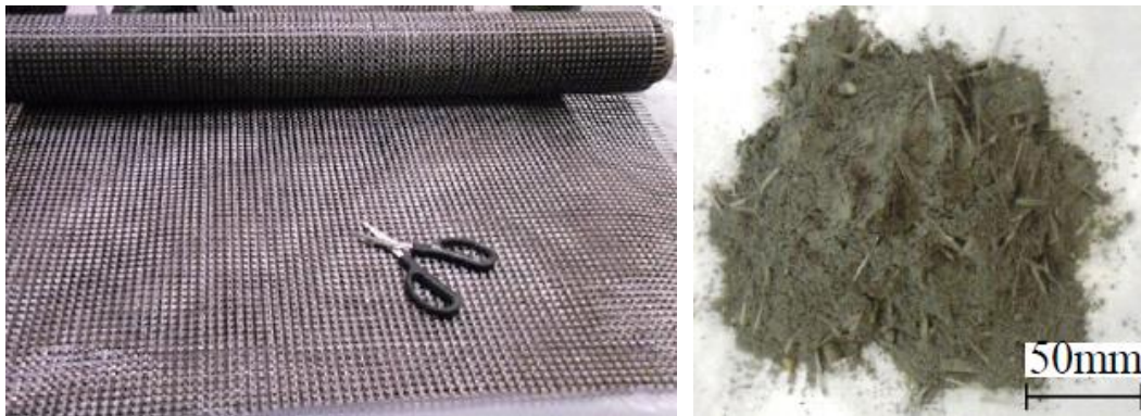
Figure 2.2 – Carbon 2 fabric roll and the inorganic cementitious mortar
