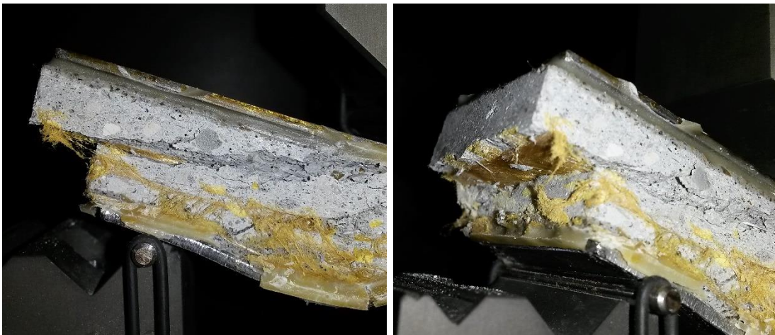
Figure 4.26 – Valid interlaminar shear failure obtained with the four-ply PBO-FRCM
