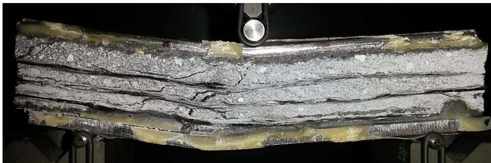
Figure 4.24 – Typical failure mode for four-ply Carbon 1-FRCM composite sandwich beam with steel facings of 4.0mm
