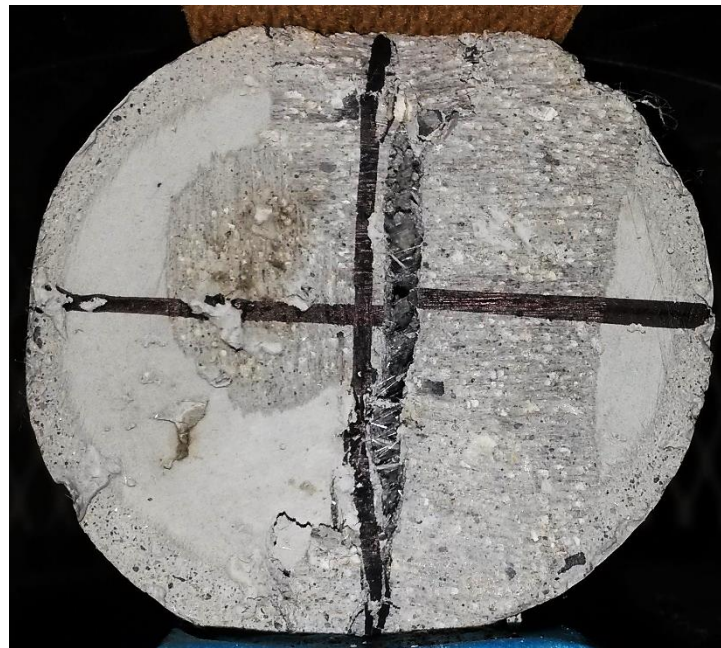
Figure 4.40 – Typical failure mode of mortar cylinders subjected to splitting tensile test
