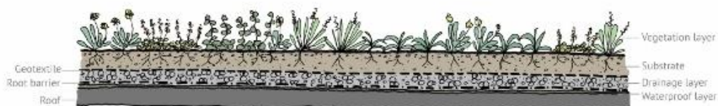
Figure 31: Green roof. (Susdrain, 2015)
