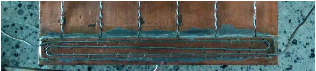
Figure 3.9: Heater brazed onto the copper plate with the Thermocoax bended in a S shape
