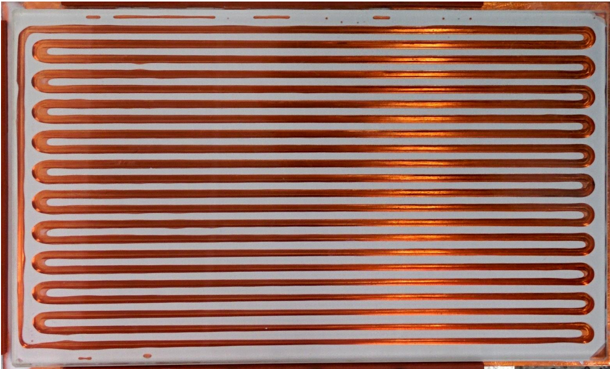
Figure 3.4: Front view of the “white” PHP with the NUSIL glue
