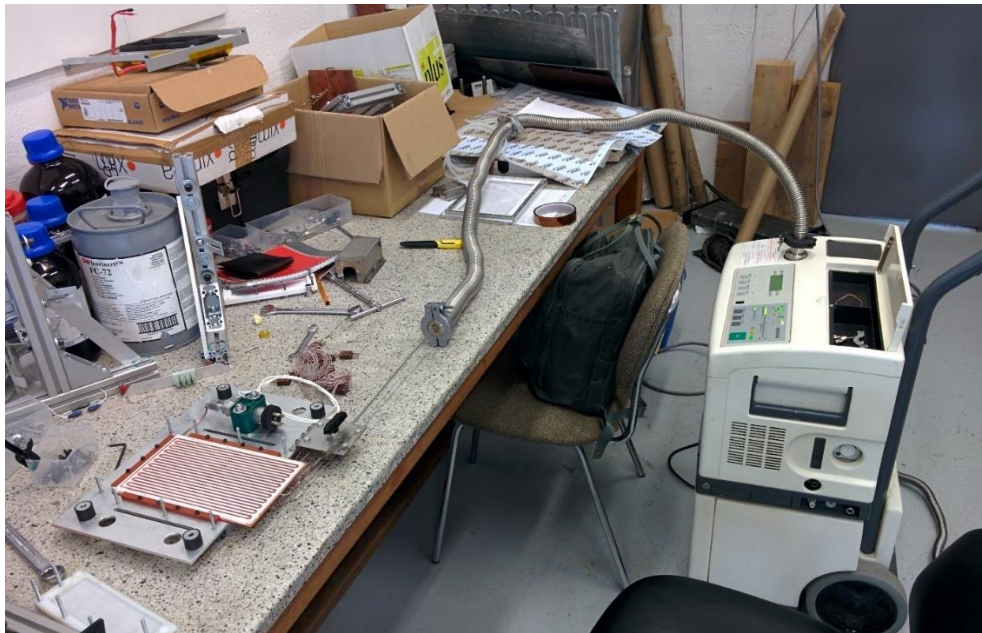
Figure 4.14: Emptying process of the PHP made with the Nusil glue
