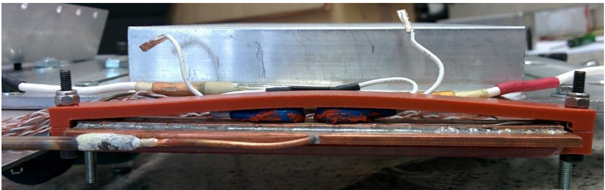
Figure 3.14: Thermal Switches (in blue) hold by the Ertalon 4.6 clamp
