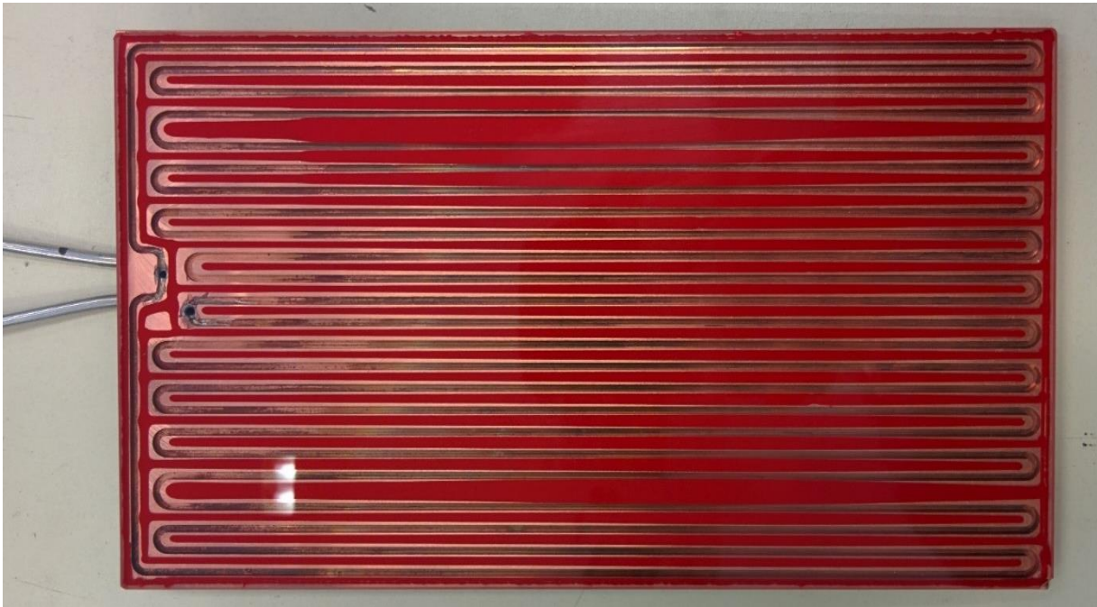
Figure 4.6: PHP after the cure of the glue. Loctite glue.
