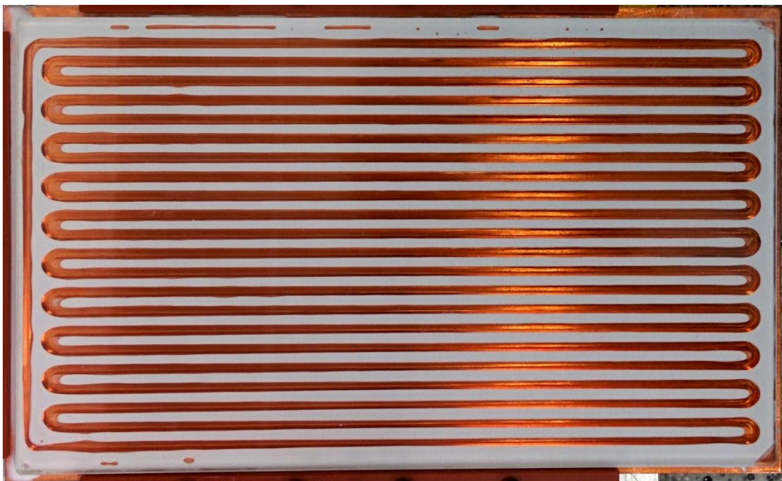
Figure 4.13: The second and definitive “white” PHP made with the Nusil glue and the primer on the copper plate.
