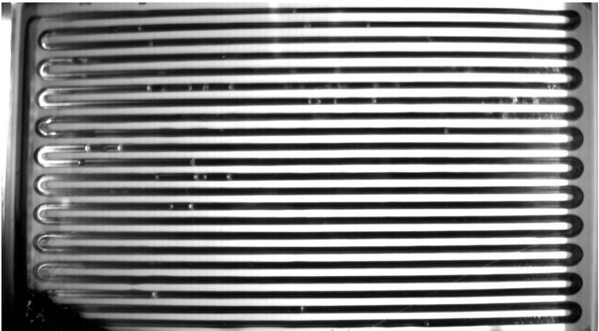
Figure 6.26: Typical flow pattern in microgravity for medium-low heat power. Frame of the parabola number 9 on the second day of parabolic flight (70W).
