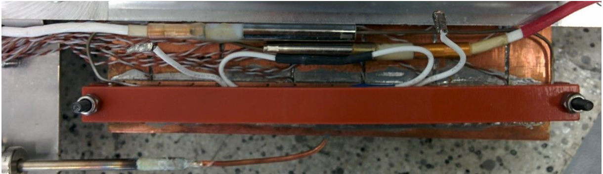
Figure 3.10: View of the heater with the two thermal switch hold by the Ertalon 4.6 clamp
