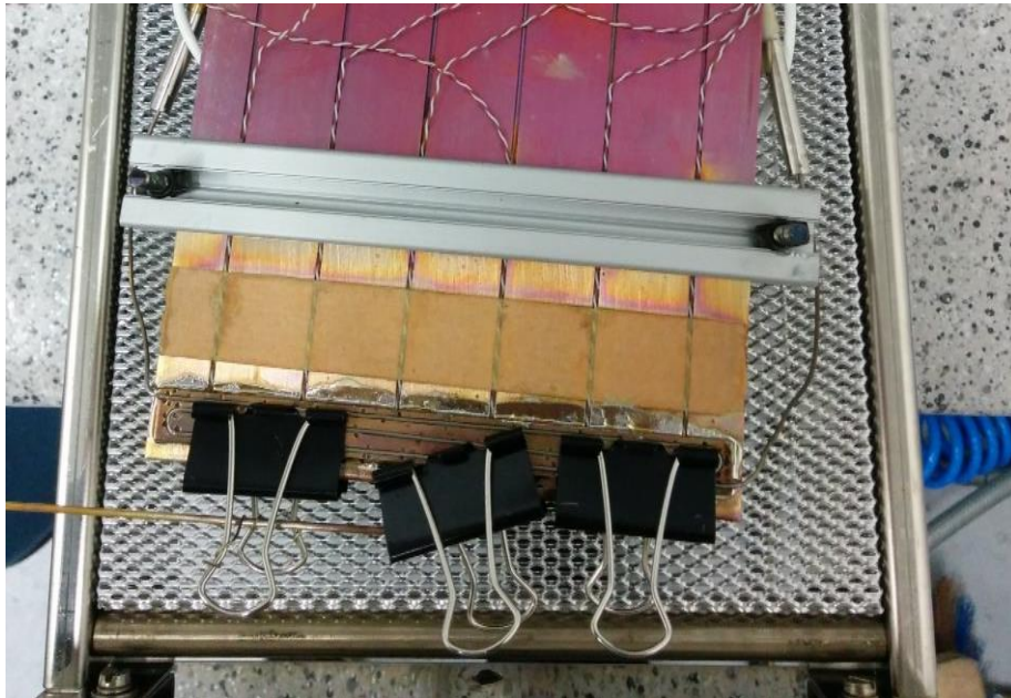
Figure 4.8: PHP just after the brazing process for the heater and the two tubes
