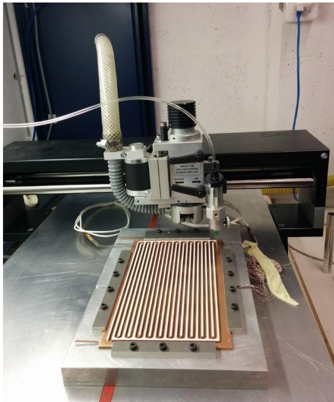
Figure 4.11: gluing process with the Nusil glue
