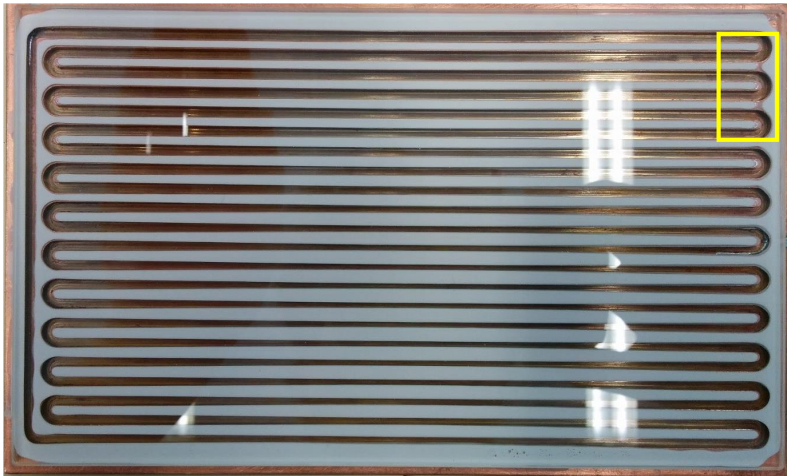
Figure 4.12: First PHP made with the Nusil glue. On the box the two little bridges on the glue
