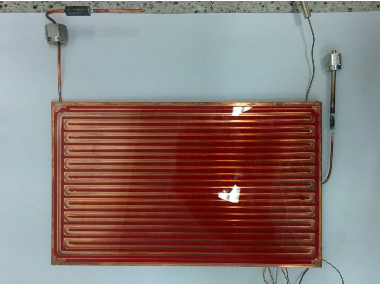
Figure 4.10: Final PHP with the Loctite glue. The Nusil Glue on the upper part of the PHP (Left on the picture) was not already placed
