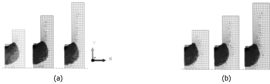
Figure 4-10 Plastic zone (grey) for constant H_2/D=4.3 and \sigma_0/S_u=6.0 with varied H_1/D . Left to right: H_1/D= 1.0, 2.0 and 3.0 respectively. (a) \phi/D=3.1 and (b) \phi/D=4.3 . RLSR=1.0.
