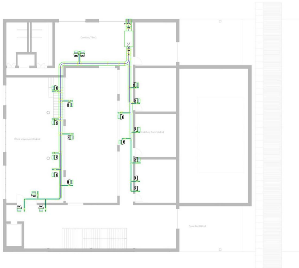
Figure 7.28 Air Conditioning System scheme in First Floor
