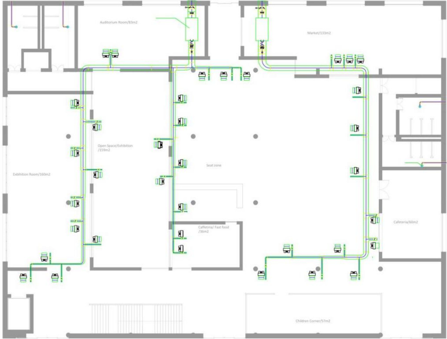
Figure 7.27 Air Conditioning System scheme in Ground Floor
