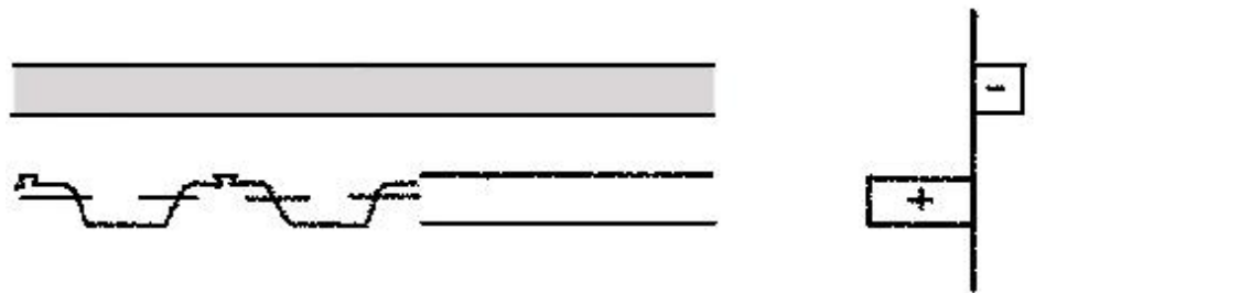
Figure 6.5 Centroid Axis of the Composite Slab
