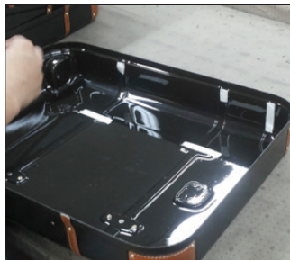
Fig.25_ Protection tape positioning
