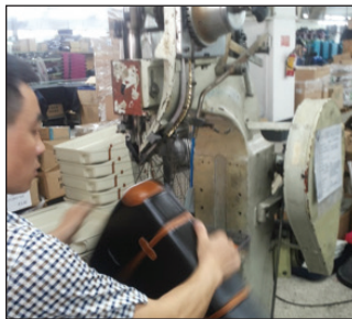
Fig.21_ Leather fixing with rivets
