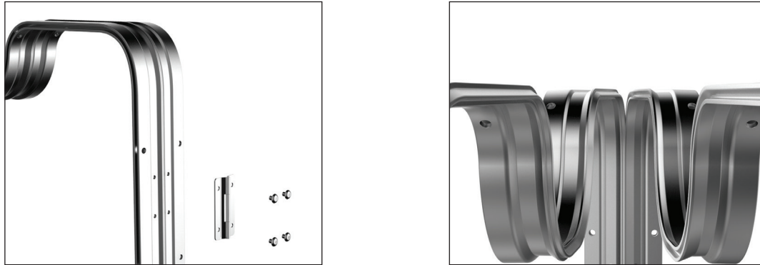
Fig.63_ Metal frame subassembly exploded views
