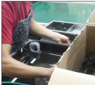
Fig.23_ Wheel fixing with self_threading screws
