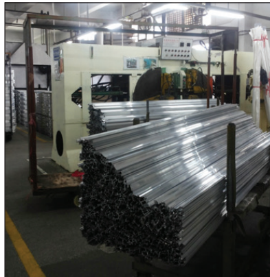
Fig.32_ Aluminium extruded profiles for metal frame
