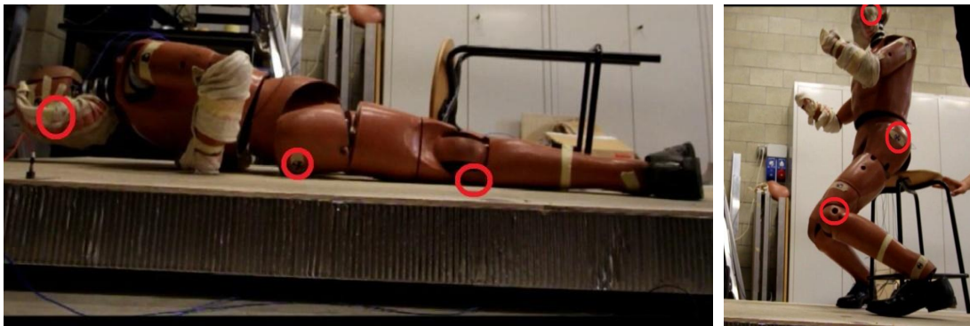
Figure 65 After fall posture (left), Figure 2. Pre-fall posture (right) with the points marked during analysis of F-0-6-0A-3-F
