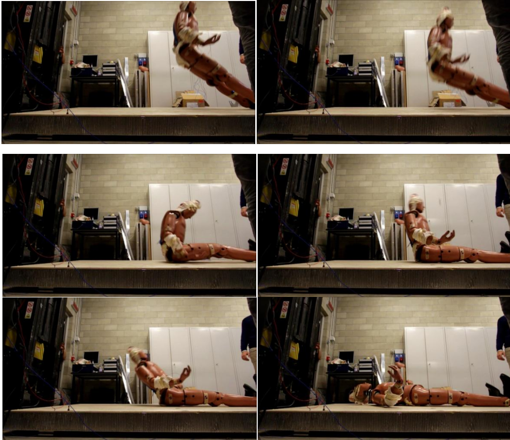
Figure 12 Frames showing postures of the dummy during a free backward fall
