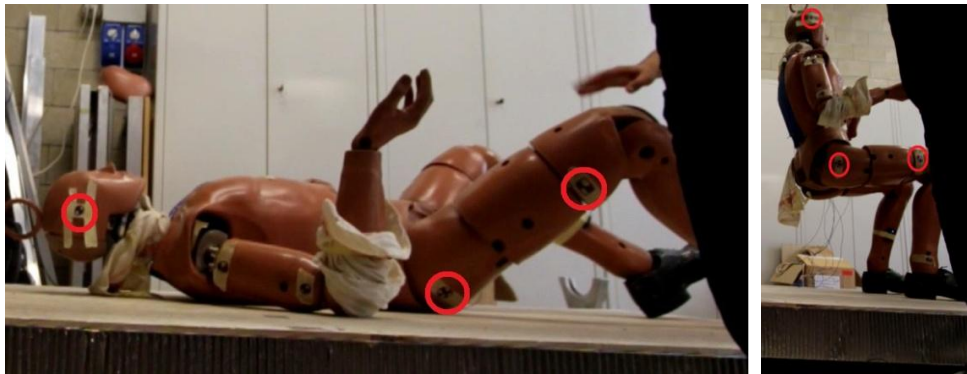
Figure 68 After fall posture (left), Figure 2. Pre-fall posture (right) with the points marked during analysis of R-1-5-0A-3-F
