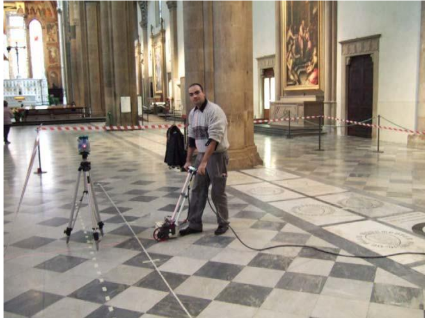
Figure 21 Georadar system in operation
