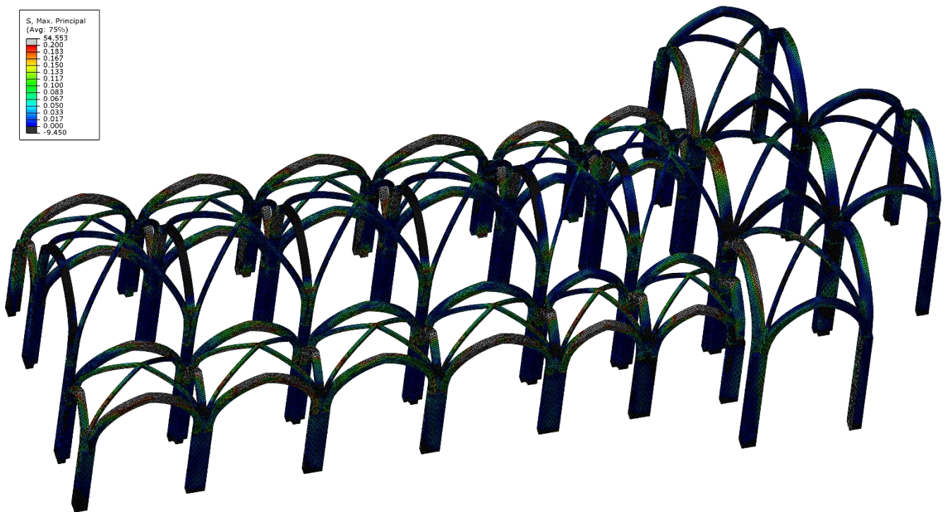
Figure 107 Maximum principal stress of the elements of arches and pillars with 20cm seeding
