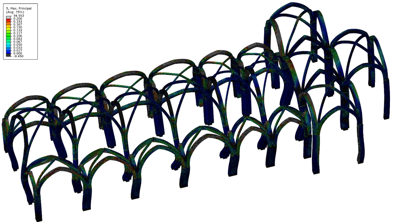
Figure 99 Maximum principal stress of the elements of arches and pillars with 20cm seeding
