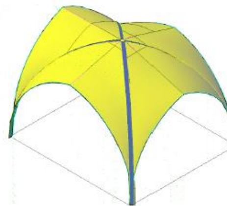
Figure 28 Creation process of the surfaces of the vaults
