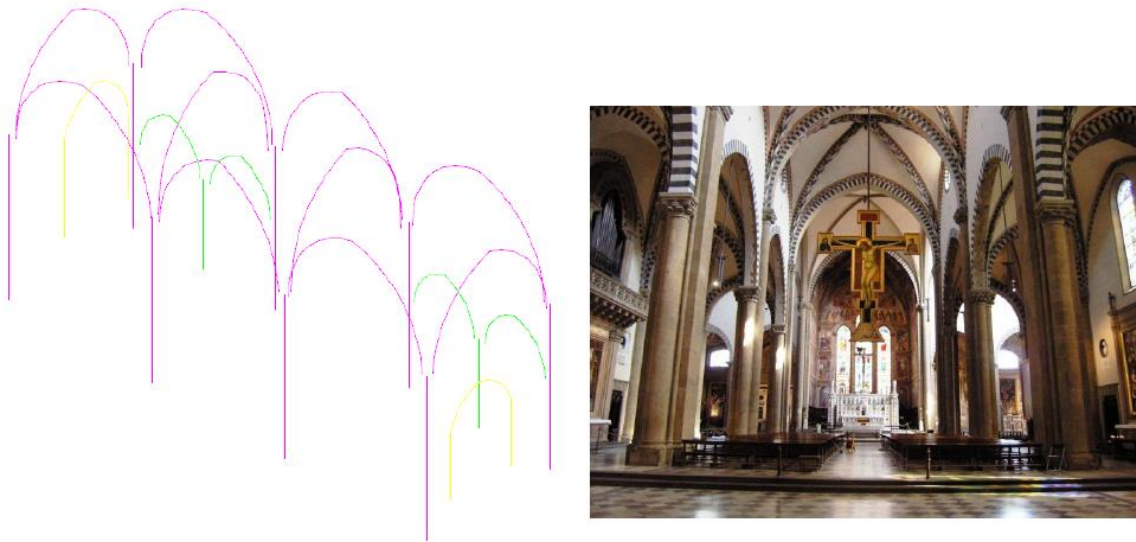
Figure 27 Mono-dimensional element (arches, ribs and pillars)
