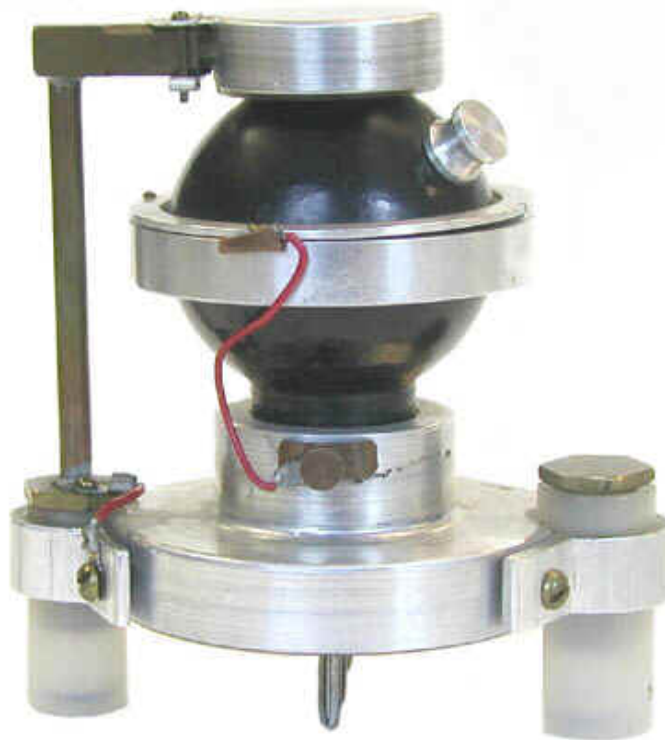
Figure 1.1: A spherical Rossi counter that was actually used by Rossi at Columbia University [8].
