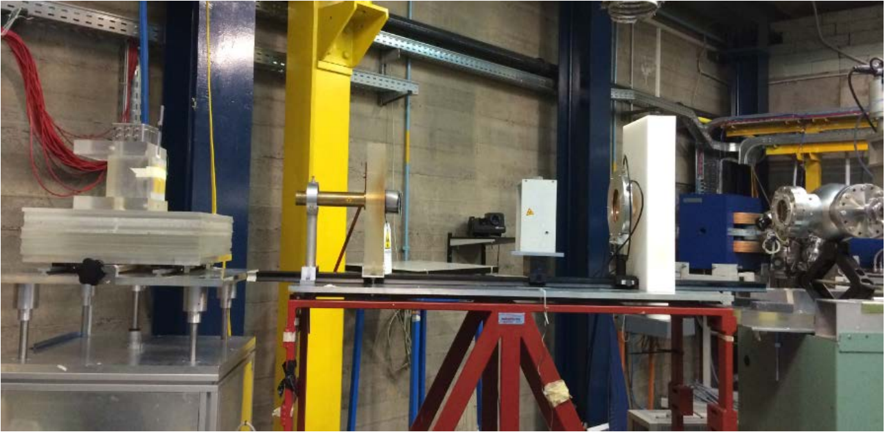
Figure 4.1: A picture of the irradiation set-up and the beam delivery system of the “Test” experimental room of CATANA facility.
