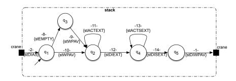
Figure 7.10: The Stack component behavior.
