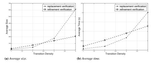
**Figure 8.9:** Average size of the automata generated and time required by the refinement and the replacement verification procedures with respect to the transition density, in the cases in which the refinement does not satisfy the property of interest.
