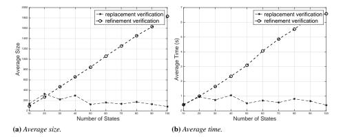
**Figure 8.6:** Average size of the automata generated and time required by the refinement and the replacement verification procedures with respect to the number of the states of the automata when the property  $\phi_1$  is considered.
