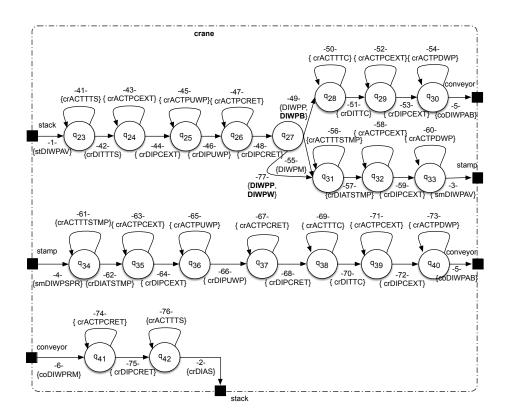
Figure 7.17: The Crane behavior proposed in the second refinement Scenario.
