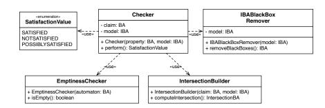
Figure 6.4: The class diagram of the CHIAChecker module.
