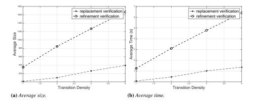
**Figure 8.5:** Average size of the automata generated and time required by the refinement and the replacement verification procedures with respect to the transition density when the property  $\phi_1$  is considered.
