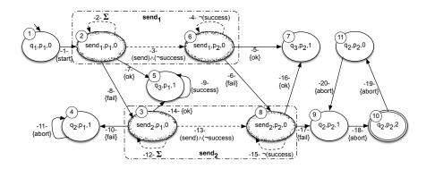
**Figure 5.2:** The intersection automaton  $\mathcal{I}$  between the incomplete BA  $\mathcal{M}$  and the BA automaton  $\overline{\mathcal{A}_{\phi}}$  which corresponds to the negation of the property  $\phi$ .
