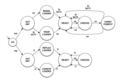
Figure 6.1: The state machine describing the behavior of the CHIA framework.
