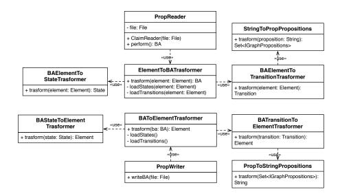
Figure 6.3: A portion of the class diagram of the CHIAAutomataIO module.
