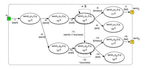
**Figure 5.7:** Intersection between the replacement  $\mathcal{R}_{send_1}$  described in Figure 5.6a and the sub-property  $\overline{S_{send_1}}$  presented in Figure 5.4a.
