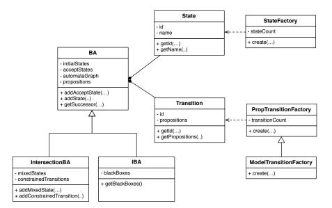
Figure 6.2: The class diagram of the CHIAAutomata module.
