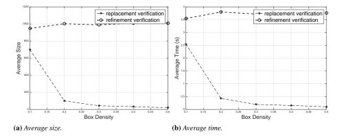
**Figure 8.8:** Average size of the automata generated and time required by the refinement and the replacement verification procedures with respect to the box density when the property  $\phi_1$  is considered.
