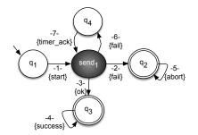
Figure 5.5: A modeling alternative for the sending message protocol example.
