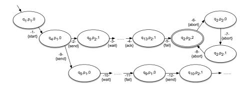
Figure 3.4: A portion of the intersection automaton obtained from the BAs specified in Figure 3.1 and 3.3, respectively.
