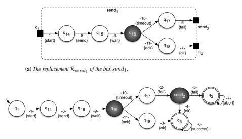
(b) The refinement  $\mathcal{N}$  obtained by plugging the replacement  $\mathcal{R}_{send_1}$  into the model  $\mathcal{M}$ .
