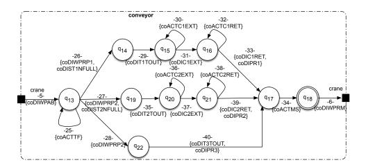
Figure 7.14: The Conveyor component behavior.
