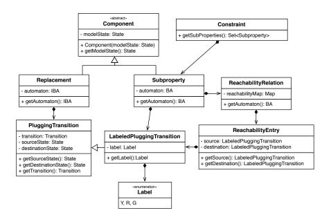
Figure 6.5: The class diagram of the CHIAConstraint module.
