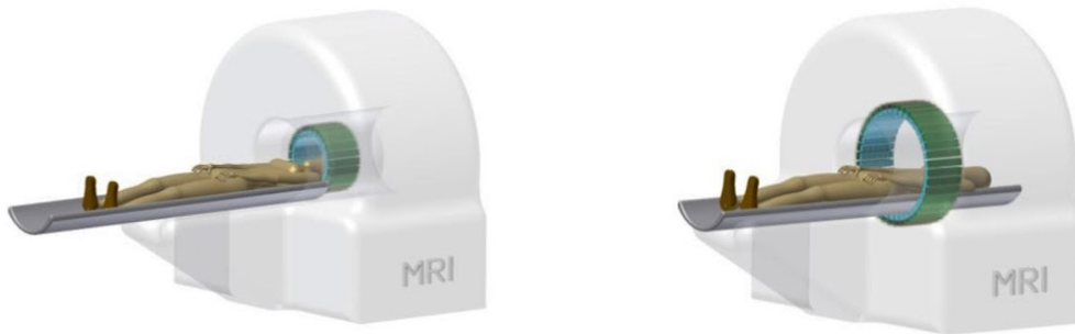
Figure 1.2: Schematic views of a synchronous, or integrated, design for combined nuclear medicine and radiology scanners. The two imaging device are integrated one inside the other. On the left, a combined PET/MRI for head/neck acquisition. On the right, a whole-body PET/MRI scanner. [7]
