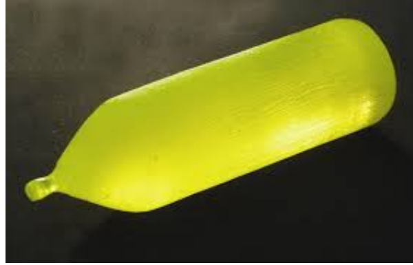
Figure 3.25: Gd_3Al_2Ga_3O_{12} (GAGG(Ce)) scintillator block from Furokawa, Japan. [117]
