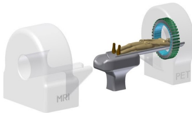
Figure 1.1: Schematic view of a sequential, or “tandem”, design for combined nuclear medicine and radiology scanners (in this example a PET/MR). The two imaging device are arranged with the gantries in the direction of the main scanner axis with a patient handling system (usually placed on a track) mounted in between. [7]
