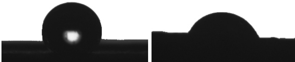
Figure 5.4: Optical pictures of drops on 4-Pa-Pr and 4-Pa-S show high contact angles suggesting hydrophobicity of the samples.
