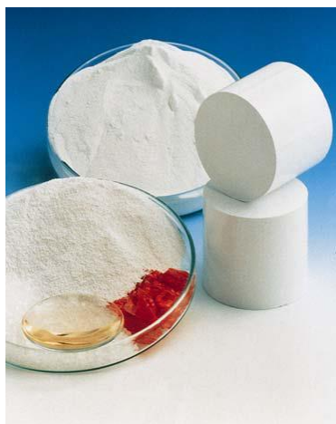
Figure 1.5 Powder of aluminum oxide ( \text{Al}_2\text{O}_3 ) with a small percentage of MgO (A. Porporati, 2014, Ceramici per articolazioni)
