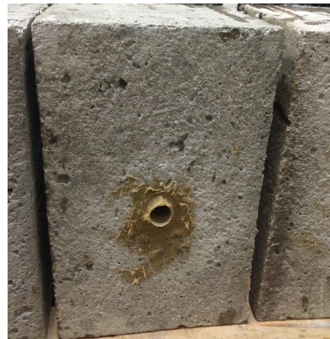
Fig. 2. 34 - Installation of the plastic tubes inside the holes (bottom view)
