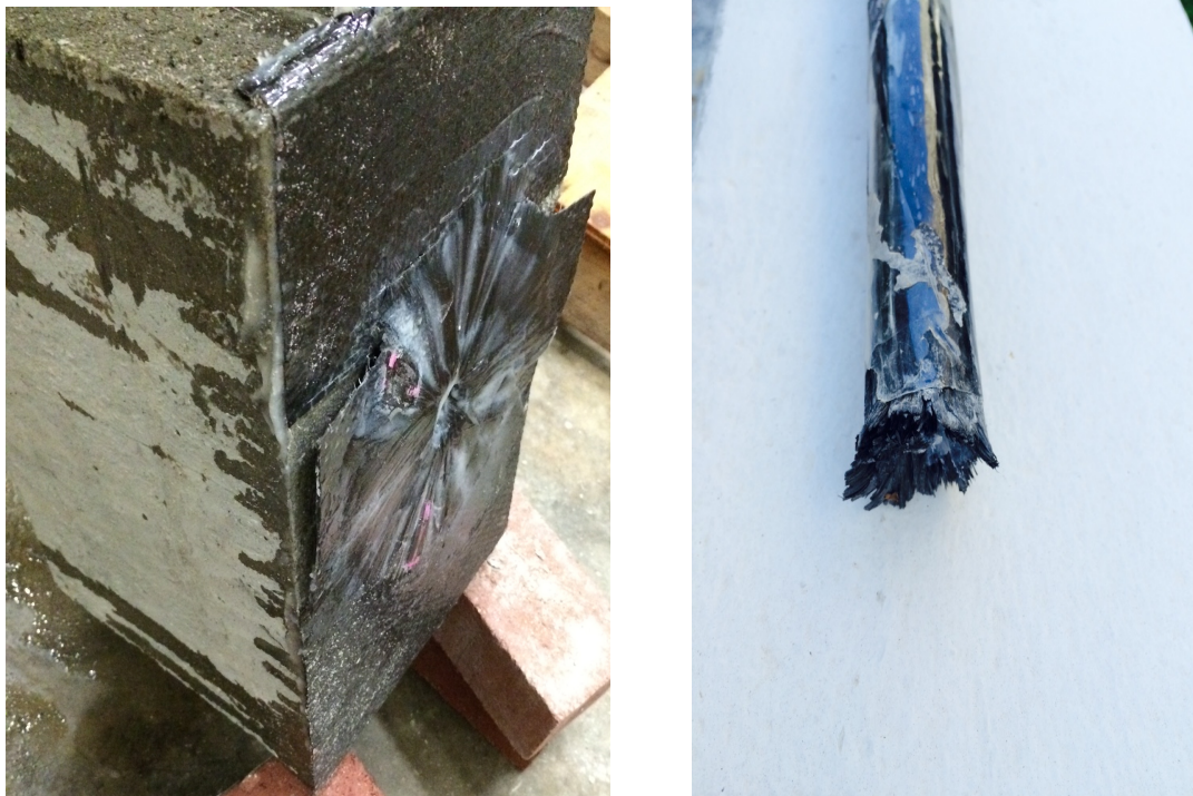
Fig. 3. 5 - FRP System (left) and Anchor Dowel (right) after the failure (Failure mode B)
