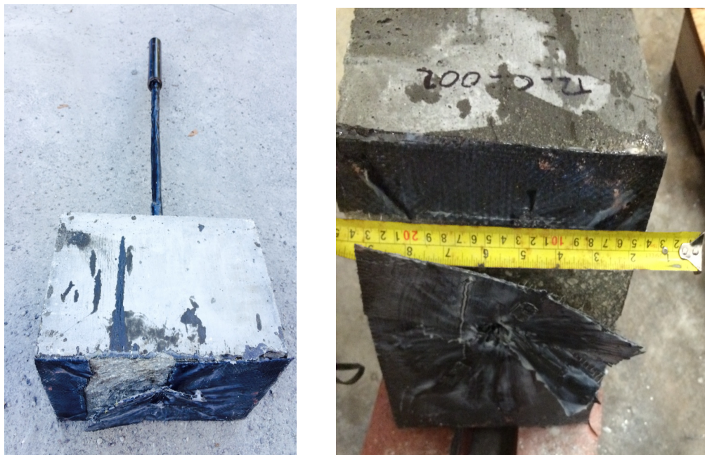
Fig. 3. 4 - Failure Mode A
