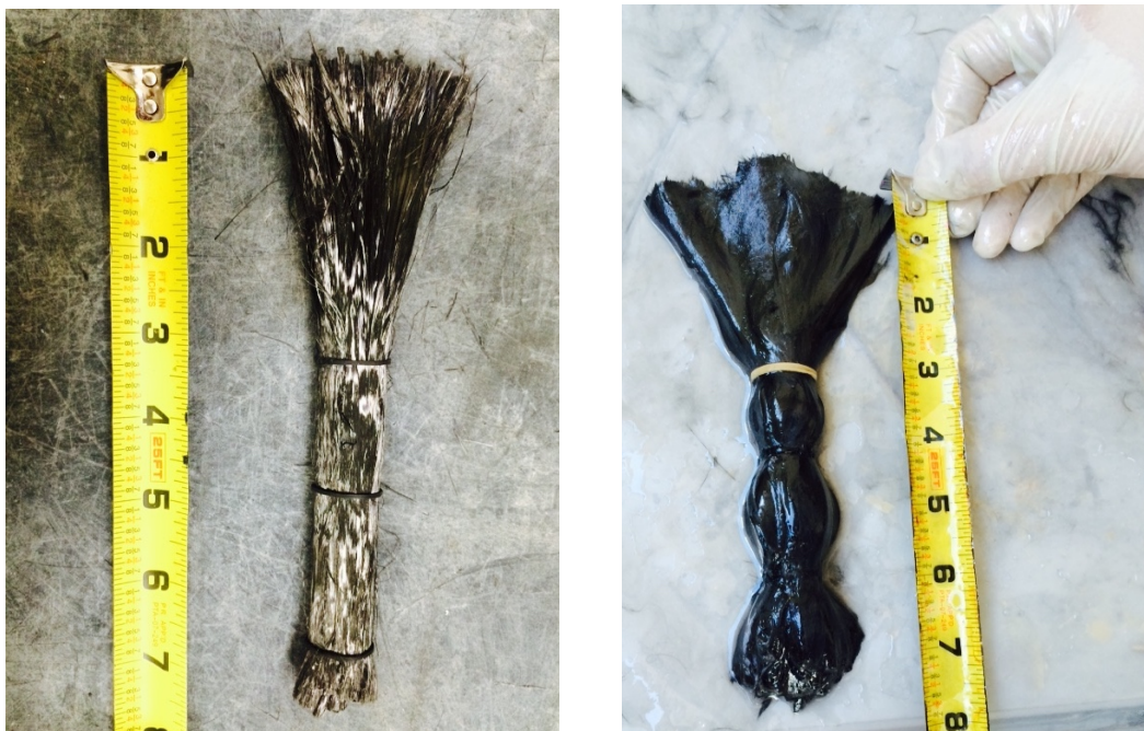
Fig. 2. 44- Anchor before (left) and after (right) the impregnation of the fibers
