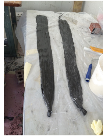
Fig. 2. 26 - Anchor after the impregnation
