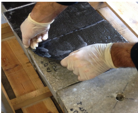
Fig. 2. 32 – Installation (left) and rolling (right) of the FRP sheet
