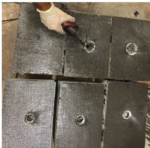
Fig. 2. 33- Operation of cutting the FRP sheets
