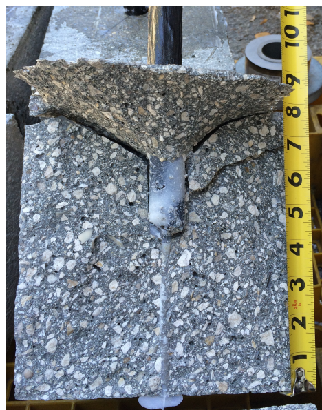
Fig.3. 2 - Failure mode B
