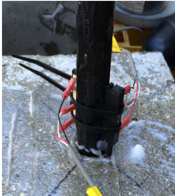
Fig. 2. 53 - Installation of the potentiometer
