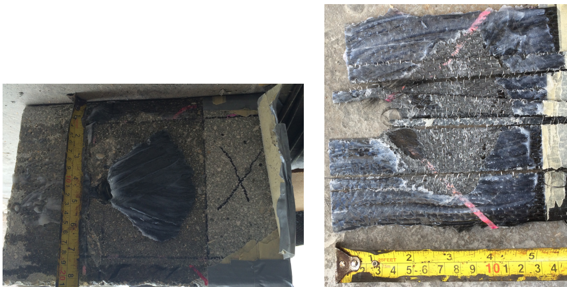
Fig. 3. 8 - Specimen (left) and FRP sheet (right) after the failure of the system (Failure Mode C)
