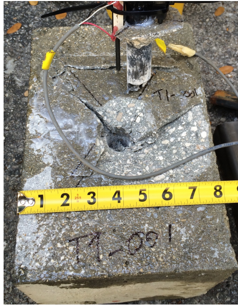
Fig. 3. 1 – Failure mode A
