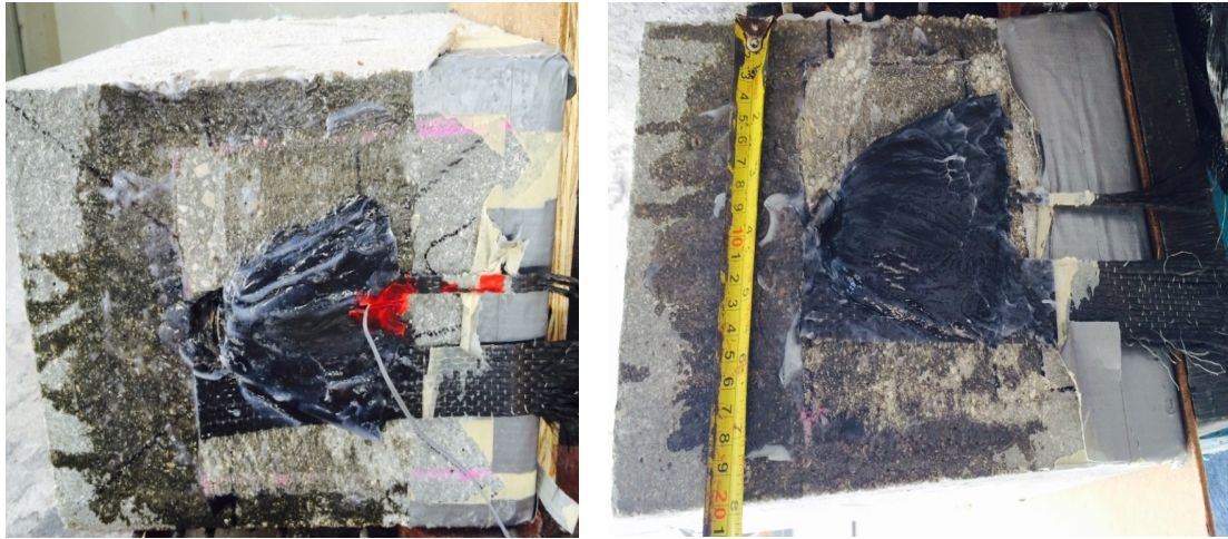
Fig. 3. 7 - Failure Mode B
