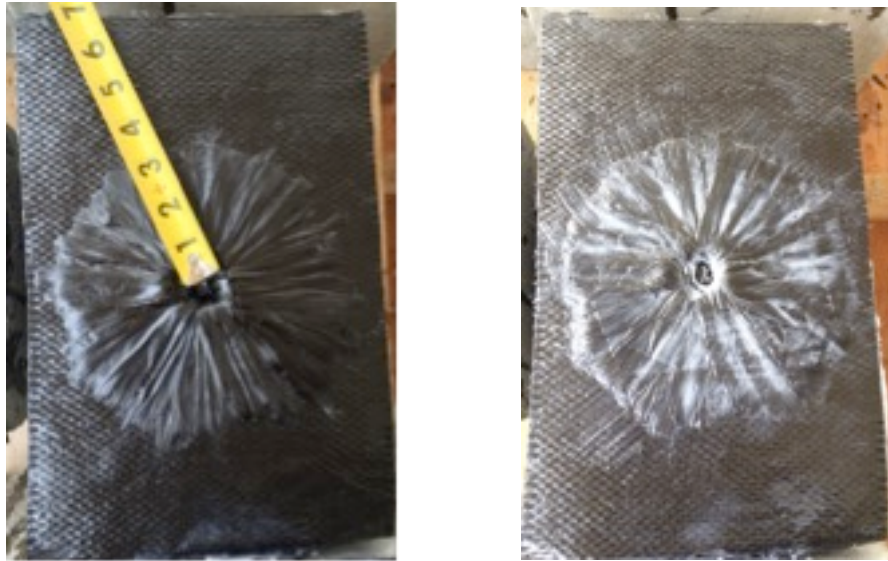
Fig. 2. 37 - Specimen before (left) and after (right) the application of the layer of thickened epoxy
