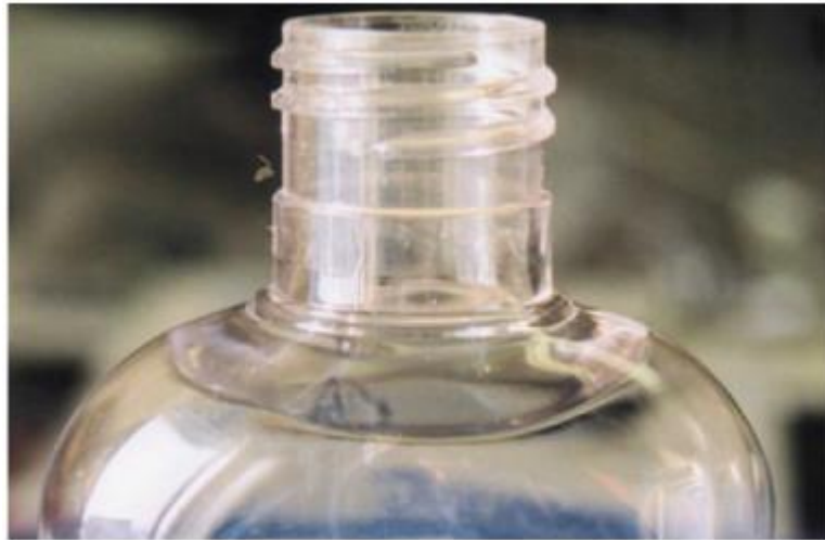
Figure 1.2 Material folding in neck area [11]
