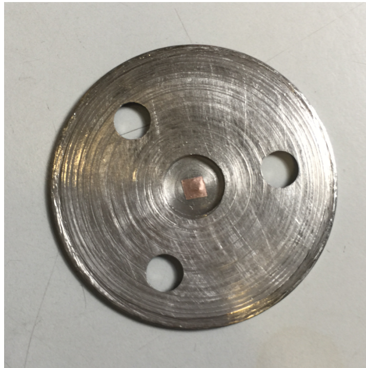
Fig.4.9. A specimen mounted on the specimen stage of the backside of cap
