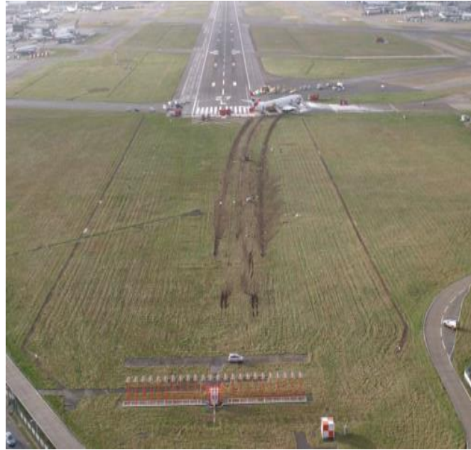
Figure 11. Boeing 777-200 operated by British Airways Landed before the Threshold, at London Heathrow Airport due to Engine failure, 17 January, 2008
