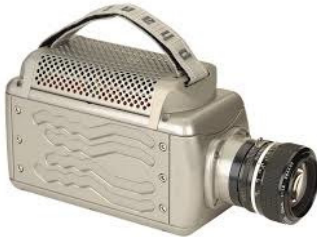
Figure 3.3: Phantom v5 used to acquire video frame.
