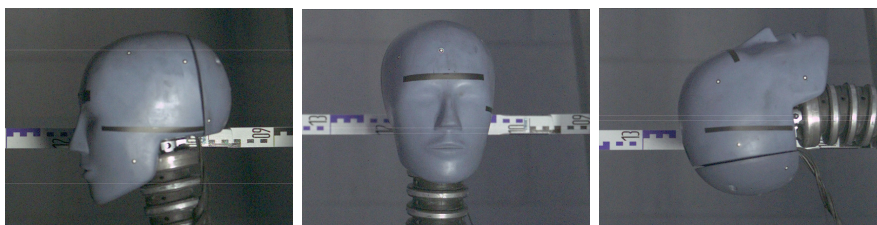
Figure 3.10: Black line in frontal impact test, configuration 1 of the inner neck cable.
