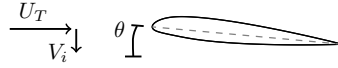
Figure 4.1: Scheme of operating conditions at a blade section: the uncertain variables are the pitch angle \theta and the induced velocity V_i . The velocity component U_T is the velocity tangential to the rotor disk.
