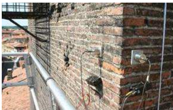
Figure 4.11 Typical external mounting of the accelerometers (01/08/2012)
