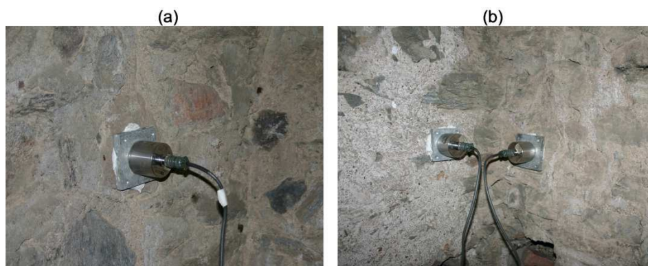
Figure 5.4 Mounting of the accelerometers at test points 7 (a) and 8-9 (b)
