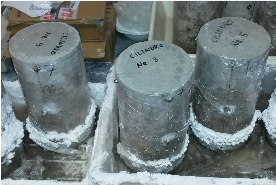
Figure 3.14: Cylinders partially immersed in 10% sodium sulfate solution after 600 days of exposure - two cylinders (left and center) are laterally wrapped while one cylinder (right) is completely wrapped
