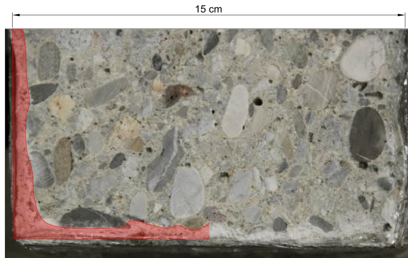
Figure 3.4: Profile of salt after 400 days on the half section of the specimen
