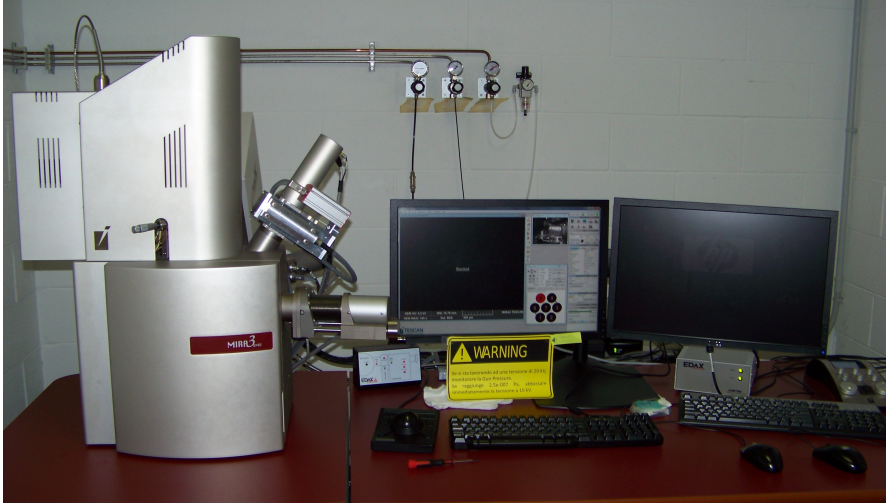
Figure 3.21: SEM-EDS MIRA3XMU - Department of Earth Sciences of the University of Pavia, courtesy of prof. Maria Pia Riccardi
