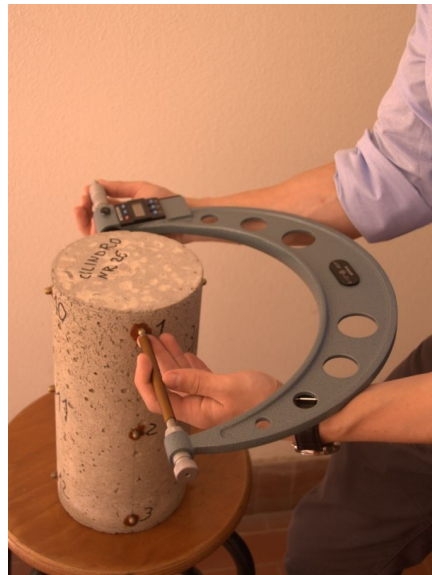
((c)) Measuring radial expansion
