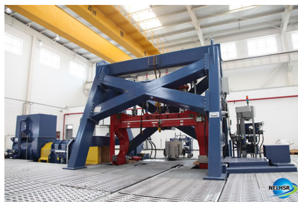
Figure 2.2: The roller rig for tests on a single wheelset at CARS.
