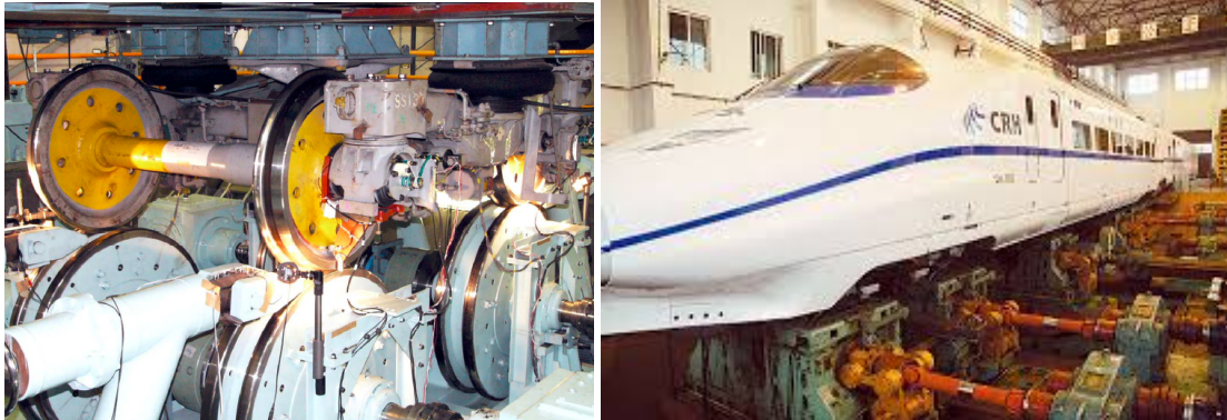
Figure 2.1: The roller rigs at NTSEL (left) [77] and SWJTU (right).
