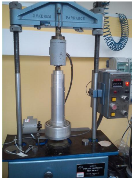
Figure 2.6. Wykeham Farrance loading frame.
