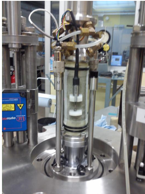
Figure 2.19. Miniature LVDT stuck to the sample measuring local axial strain.
