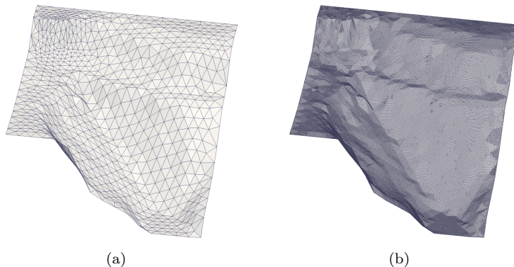
Figure 7.4: Sliding surfaces of Greenhills Cougar 7 dump. Original data (a) and the set of points used for the numerical simulation (b).
