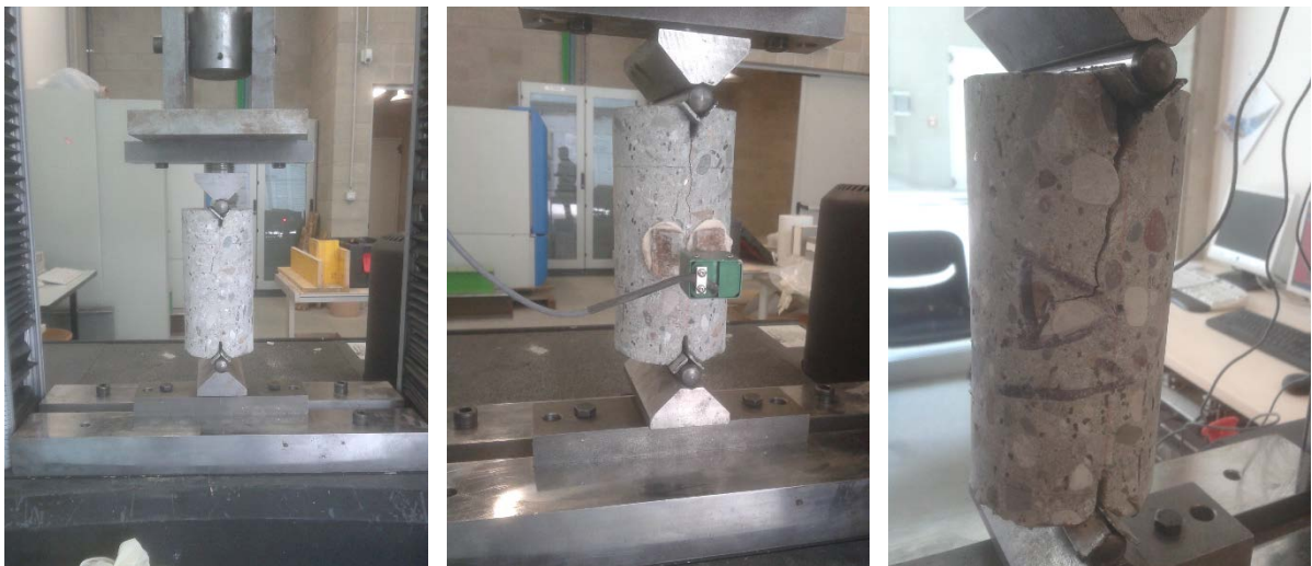
Figure 58 –Indirect tensile DEWS test in cylindrical specimen.
