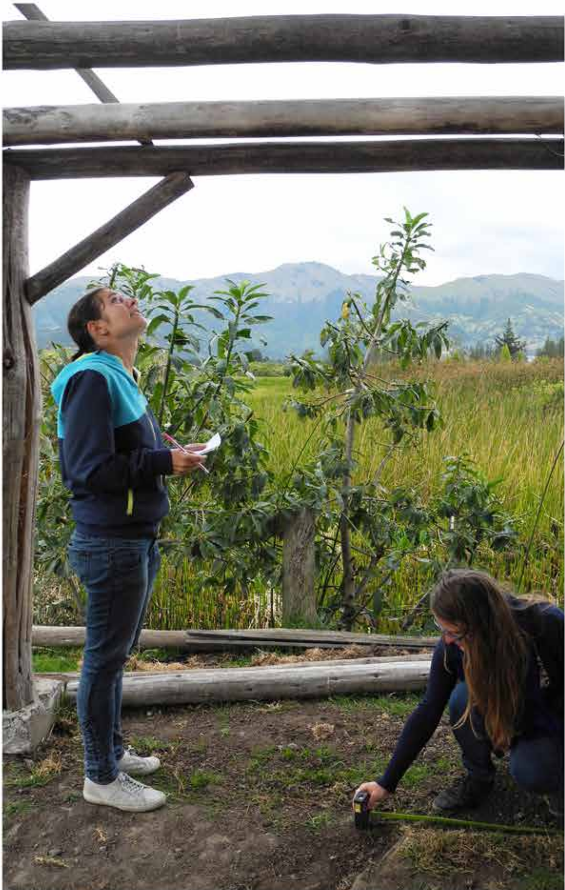
Photo: Measurement of the wooden structure height and roof inclination
