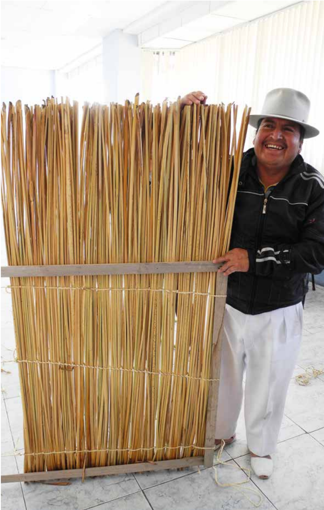
Photo: José showing the best prototype of totora wall, San Rafael de la Laguna.
