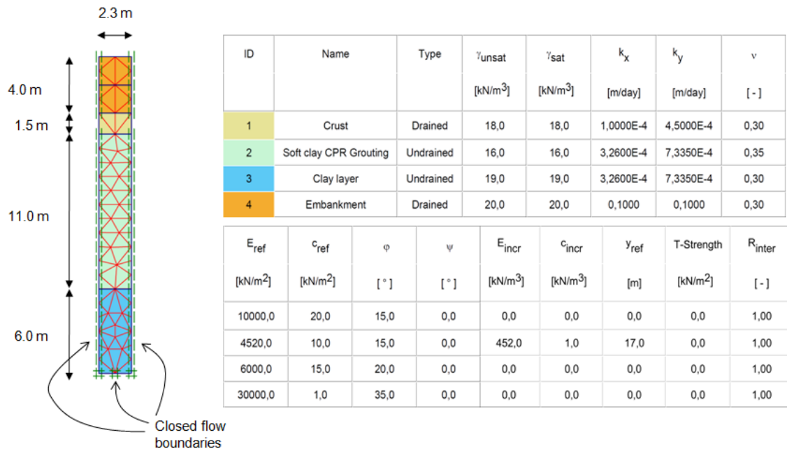
Figure 8.3: Unit cell model used in the present study for FEM analysis.
