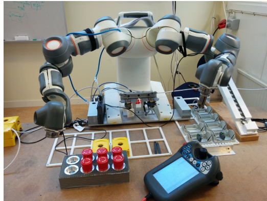
Figure 1.1: The ABB YuMi robot in the Robotics Lab of Lund University used for the experiments.
