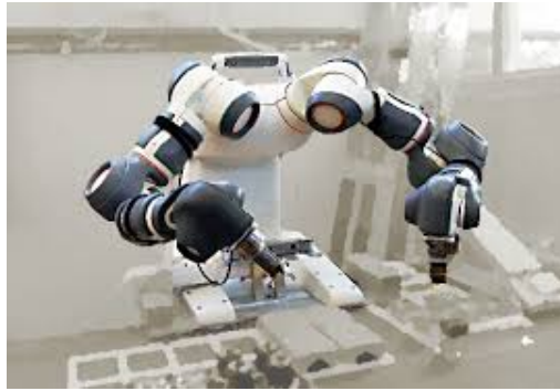
Figure 7.1: The ABB YuMi robot in the Robotics Lab used in the experimental tests.
