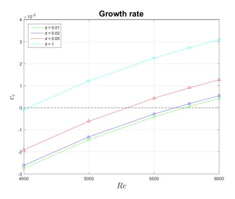
Figure 5.8: Growth rate of the most unstable eigenvalue as a function of the Reynolds number for several roughness values. Triangular grooves.  $\kappa = 1.02$ .
