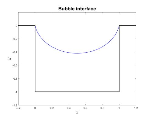
Figure 3.2: Bubble interface visualized inside a groove of unitary span.
