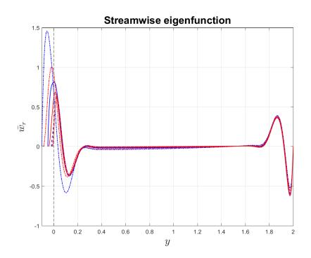
Figure 5.12: Profile of the normalized streamwise component  $\bar{w}_r$  taken at the midspan line of the section. Rectangular grooves (blue) and triangular grooves (red). Roughness d = 0.01 (dotted line), d = 0.02 (dashed line), d = 0.05 (solid line), d = 0.1 (dashed-dotted line). The black dashed line shows the groove-tip height.
