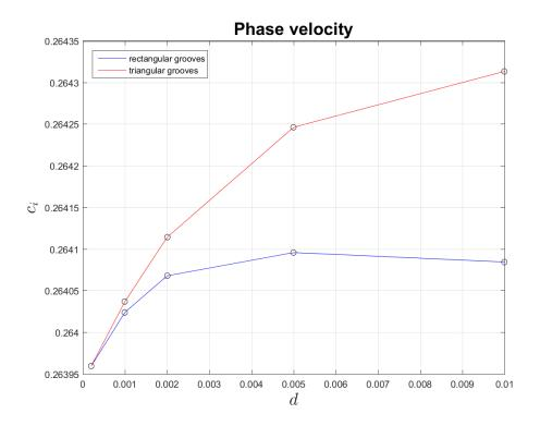
Figure 5.4: Phase speed of the dominant eigenvalue as a function of the wall roughness. Re = 5772 and  $\kappa = 1.02$ .
