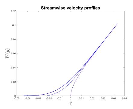
Figure 5.27: Magnification of the velocity profiles near the grooved wall (triangular grooves). Comparison between the single-phase flow (red) and the multi-phase flow (blue). Profiles taken at station V (solid line), station E (dashed-dotted line) and station T (dotted line).
