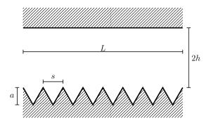
Figure 2.4: Geometric parameters of a channel with triangular grooves.
