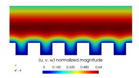
(b) Magnification near the grooves in the domain -d < y < 3d. The represented area is highlighted by a rectangle in figure 5.14a.
