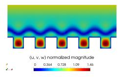
(b) Magnification near the grooves in the domain -d < y < 3d. The represented area is highlighted by a rectangle in figure 5.16a.
