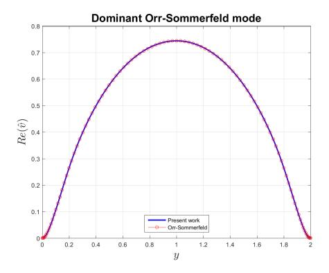
Figure 4.7: Comparison of the real part of the eigenfunction  $\hat{v}$  computed with the Orr-Sommerfeld software and the software developed for the present work.
