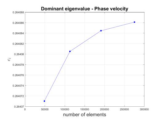
Figure 4.12: Value of the phase velocity of the dominant eigenvalue computed with different meshes.
