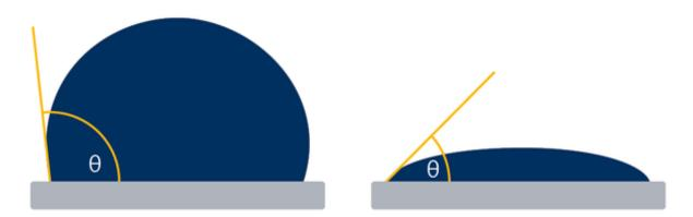
Figure 1.3: Contact angle for different surfaces. Hydrophobic surface  $\theta > 90^{\circ}$ , hydrophilic surface  $\theta < 90^{\circ}$ .
