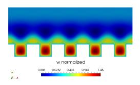
(e) Streamwise component  $\bar{w}_r$ . Rectangular grooves d = 0.1.
