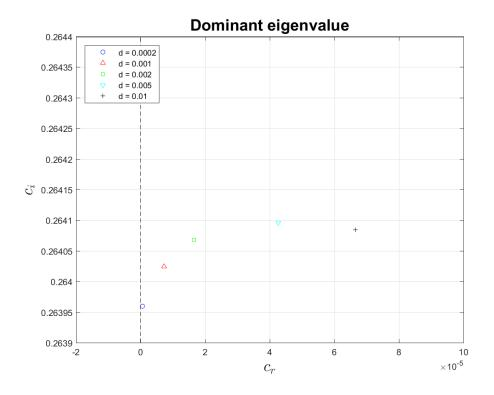
Figure 5.1: Dominant eigenvalue for rectangular grooves of different amplitude and  $\lambda = 0.02$ . Re = 5772 and  $\kappa = 1.02$ .
