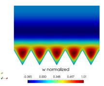
(f) Streamwise component  $\bar{w}_r$ . Triangular grooves d = 0.1.
