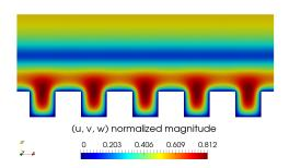
(b) Magnification near the grooves in the domain -d < y < 3d. The represented area is highlighted by a rectangle in figure 5.15a.
