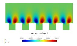
(a) Spanwise component  $\bar{u}_r$ . Rectangular grooves d = 0.1.
