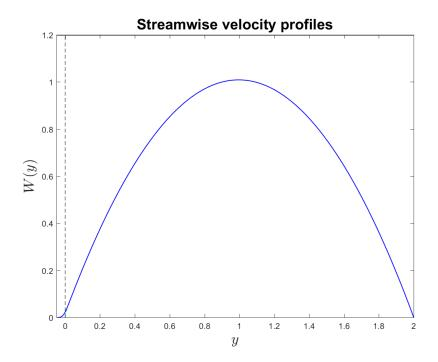
Figure 5.25: Velocity profiles in a channel with SH triangular grooves. Profiles taken at station V (blue solid line) and station T (cyan dashed line). The black dashed line shows the grooves tip height.
