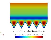
(b) Magnification near the grooves in the domain -d < y < 3d. The represented area is highlighted by a rectangle in figure 5.20a.
