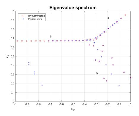
Figure 4.6: Comparison of the eigenvalues spectrum computed with the Orr-Sommerfeld software and the software developed for the present work.
