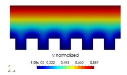
(c) Wall-normal component  $\bar{v}_r$ . Rectangular grooves d = 0.1.
