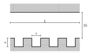
Figure 2.3: Geometric parameters of a channel with rectangular grooves.
