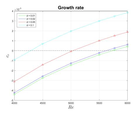
Figure 5.7: Growth rate of the most unstable eigenvalue as a function of the Reynolds number for several roughness values. Rectangular grooves.  $\kappa = 1.02$ .
