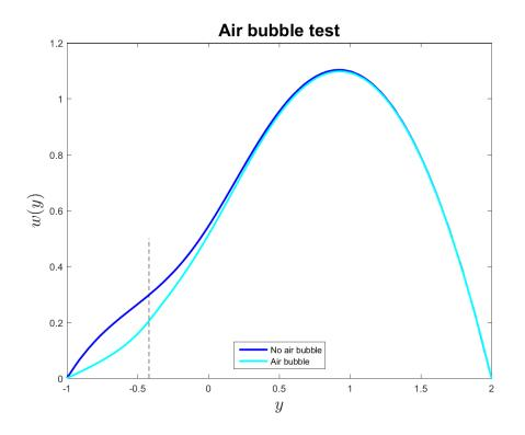
Figure 4.5: Comparison between the velocity profiles of the water flow without air bubble and with air bubble. The black dashed line shows the interface location.
