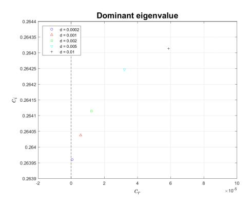
Figure 5.2: Dominant eigenvalue for triangular grooves of different amplitude and  $\lambda = 0.01$ . Re = 5772 and  $\kappa = 1.02$ .
