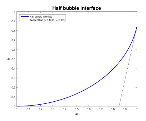
Figure 3.1: Solution for half of the groove obtained with the *Mathematica* software.
