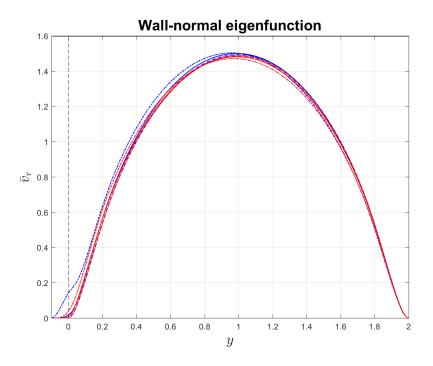
Figure 5.11: Profile of the normalized wall-normal component  $\bar{v}_r$  taken at the midspan line of the section. Rectangular grooves (blue) and triangular grooves (red). Roughness d = 0.01 (dotted line), d = 0.02 (dashed line), d = 0.05 (solid line), d = 0.1 (dashed-dotted line). The black dashed line shows the groove-tip height.
