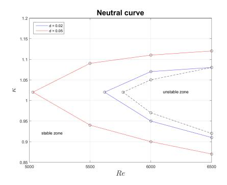
Figure 5.9: Neutral curve in the  $(Re - \kappa)$  plane for rectangular grooves of roughness d = 0.02 and d = 0.05. The black dashed line represents the approximate neutral curve of the channel with smooth walls.
