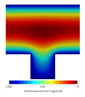
Figure 4.3: Solution to the Poisson equation for the water flow computed in two subdomains.
