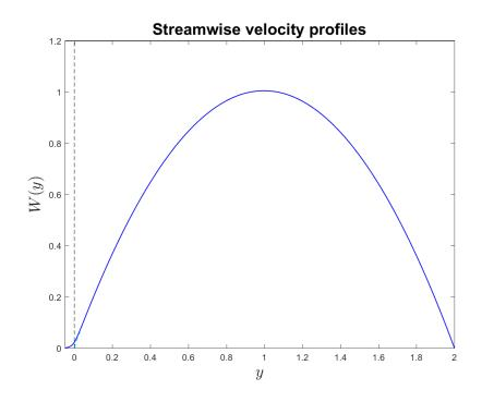
Figure 5.24: Velocity profiles in a channel with SH rectangular grooves. Profiles taken at station V (blue solid line) and station T (cyan dashed line). The black dashed line shows the grooves tip height.
