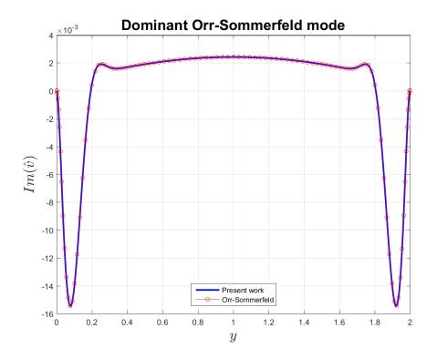
Figure 4.8: Comparison of the imaginary part of the eigenfunction  $\hat{v}$  computed with the Orr-Sommerfeld software and the software developed for the present work.
