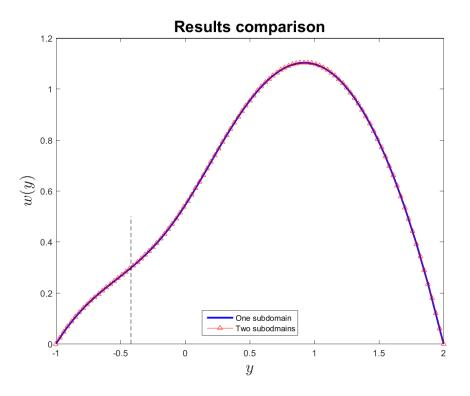
Figure 4.4: Comparison between the velocity profiles of the water flow in the grooved channel obtained with a single or two subdomains. The black dashed line shows the fake interface location.
