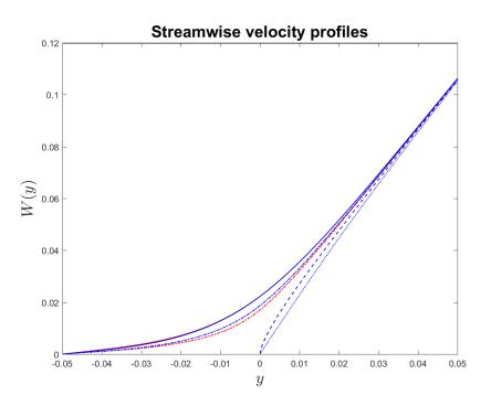
Figure 5.26: Magnification of the velocity profiles near the grooved wall (rectangular grooves). Comparison between the single-phase flow (red) and the multi-phase flow (blue). Profiles taken at station V (solid line), station H (dashed-dotted line), station E (dashed line) and station T (dotted line).
