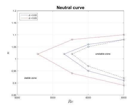
Figure 5.10: Neutral curve in the  $(Re - \kappa)$  plane for triangular grooves of roughness d = 0.02 and d = 0.05. The black dashed line represents the approximate neutral curve of the channel with smooth walls.
