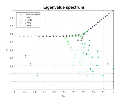
Figure 4.9: Eigenvalue spectra computed with different channel-section widths. Shift  $\xi_A$  and k = 100.
