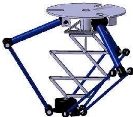
Figure 1.4: Parallel kinematic manipulator plus the coordinate measuring arm
