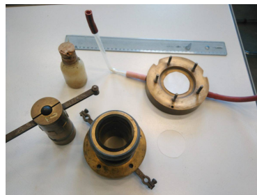
(c) Filter paper on the porous stone and gasket sealing the space between the body of the cell and the basis.
