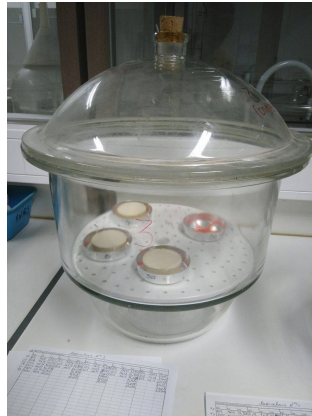
Figure 3.6: Desiccator with three samples and an empty cup (picture by Sara Rozzoni)
