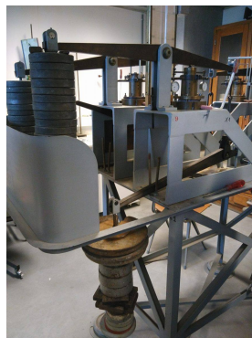
(g) Oedometric compaction - two dial gauges measure displacements.
