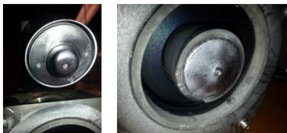
Figure 5.1: Cathode and falling insulation
