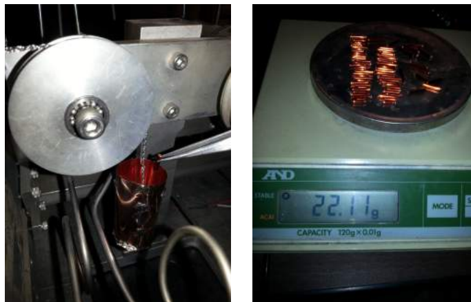
Figure 2.26: Calibration cup (left) and scale with the weights (Right)
