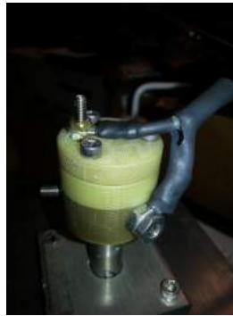
Figure 4.6: BNC Connection to the tungsten sensor
