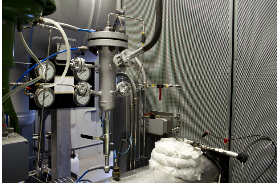
Figure 35: Picture of the constructed seeding system.
