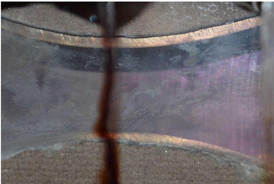
(c) Particular of the throat fouled by seeding particles.
