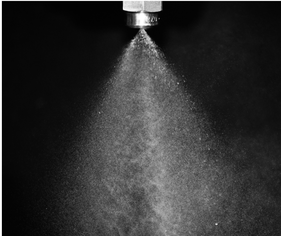
Figure 36: Picture of the spray generated by the atomizer.
