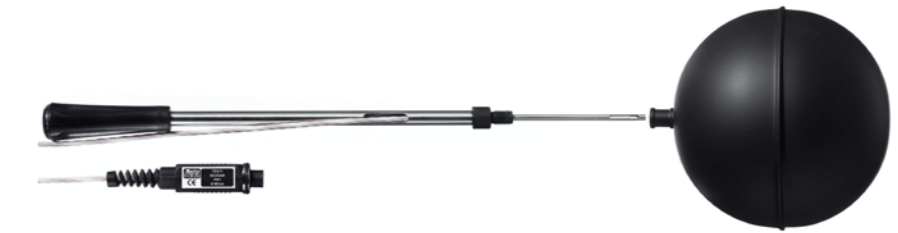
Figura 6.5 Termometro a globo
