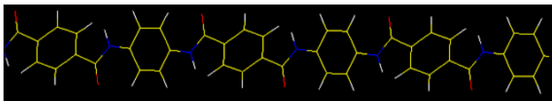
Figure 4.33- PPTA infinite single chain (1D crystal)
