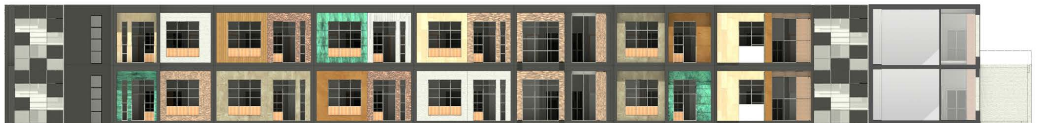
Possibility of increase the surface of the ward floor with cantilevered system
