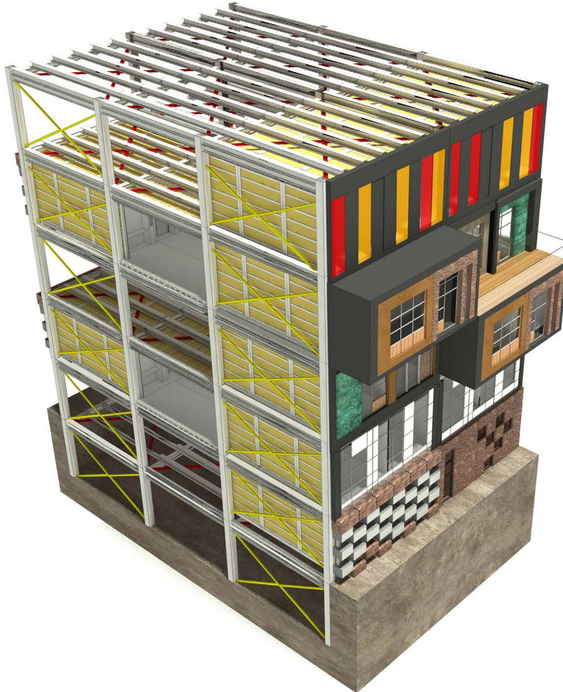
3D scheme of assembling modules into hospital building
