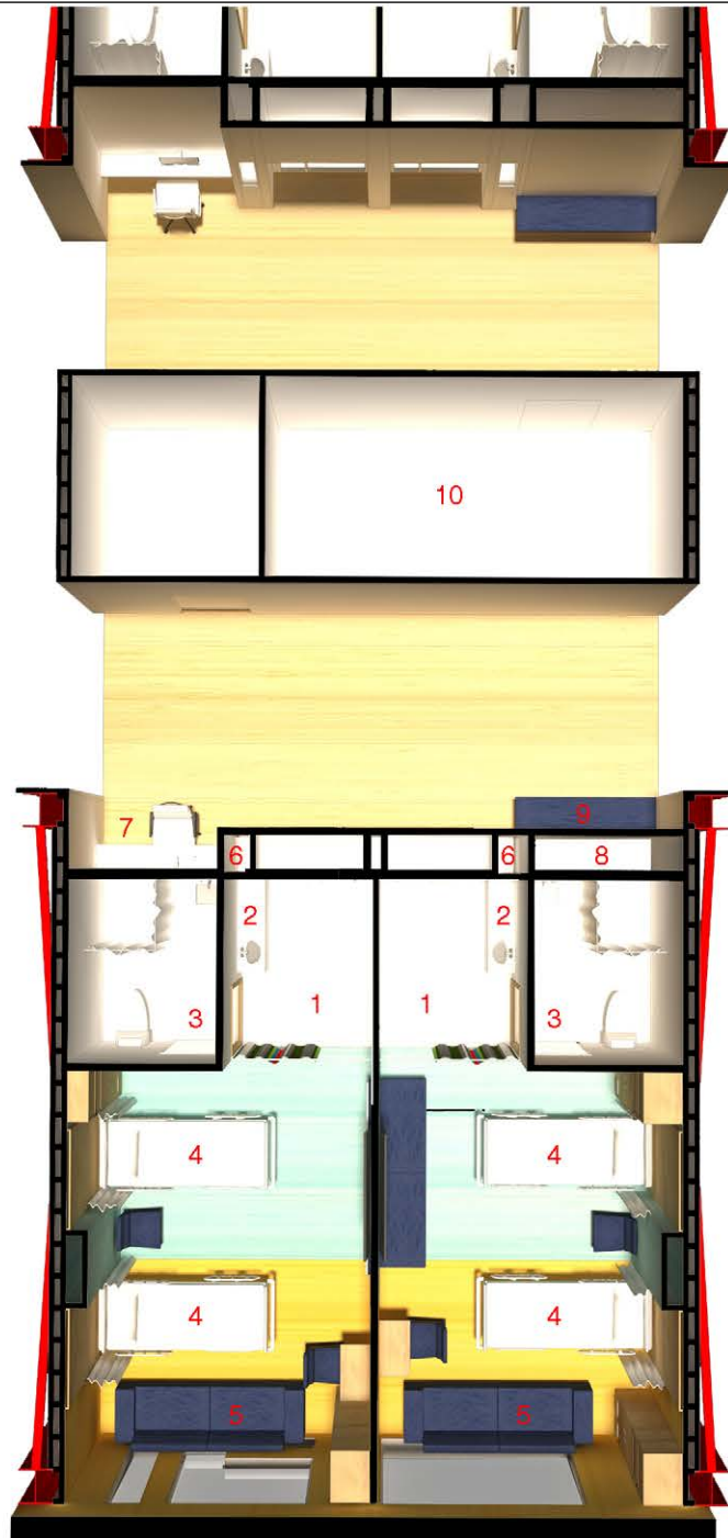
Two 2-patient wards with personnel support facilities in corridor which are also part of prefabricated module
