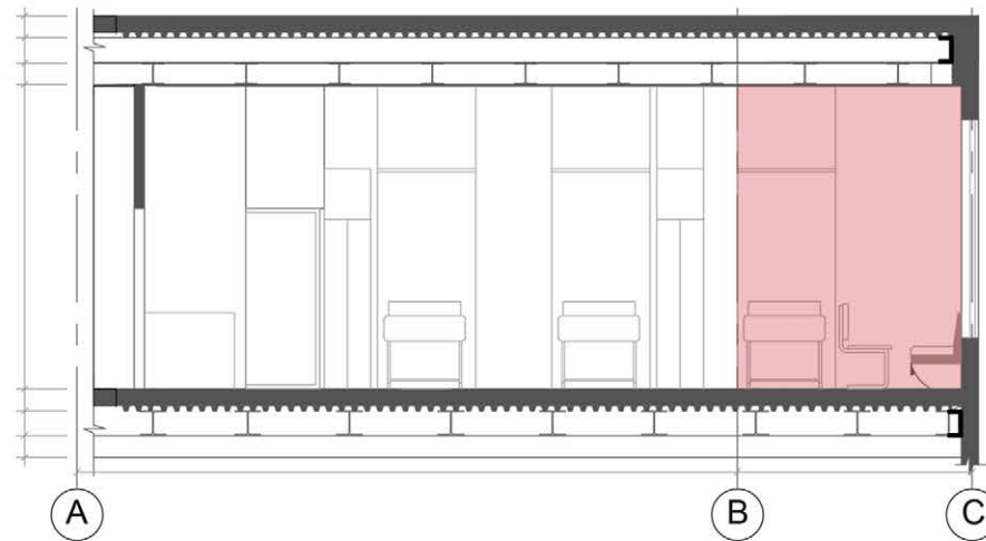
Inreasing the surface area of the module by hanging 1/3 part of prefabricated module on the facade as cantilever
