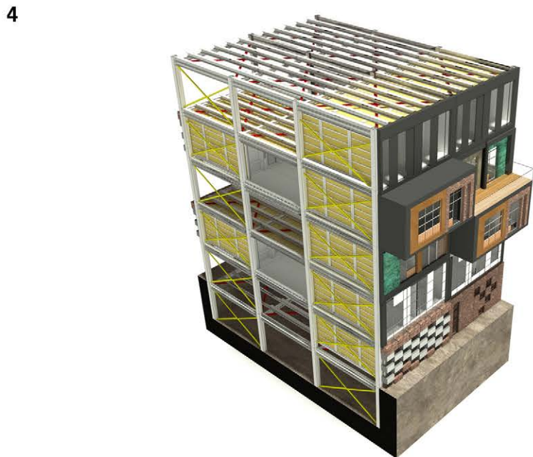
Inserting of prefabricated modules into primary skeleton
