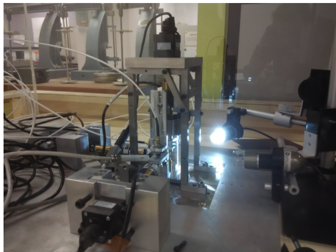
Figure 3.6: Digital micro-cameras (after Nardelli, 2014)
